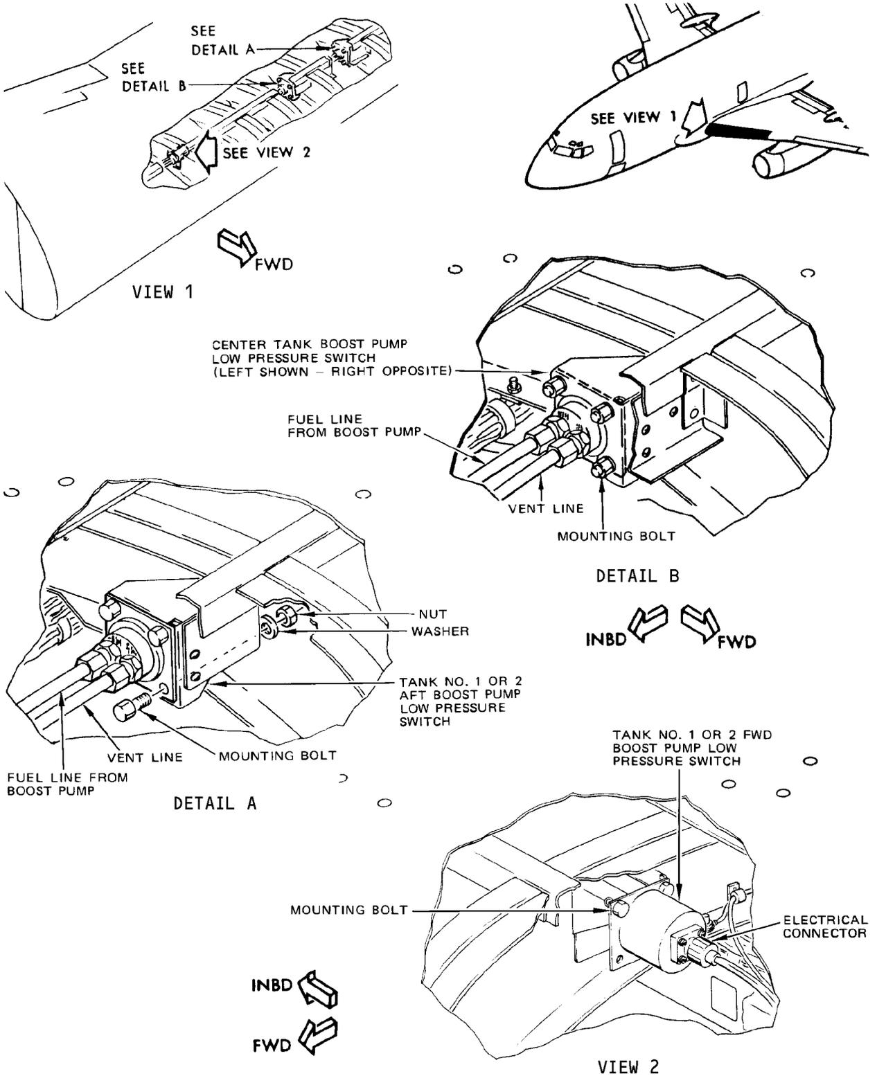
Fuel Low Pressure Switch Installation
