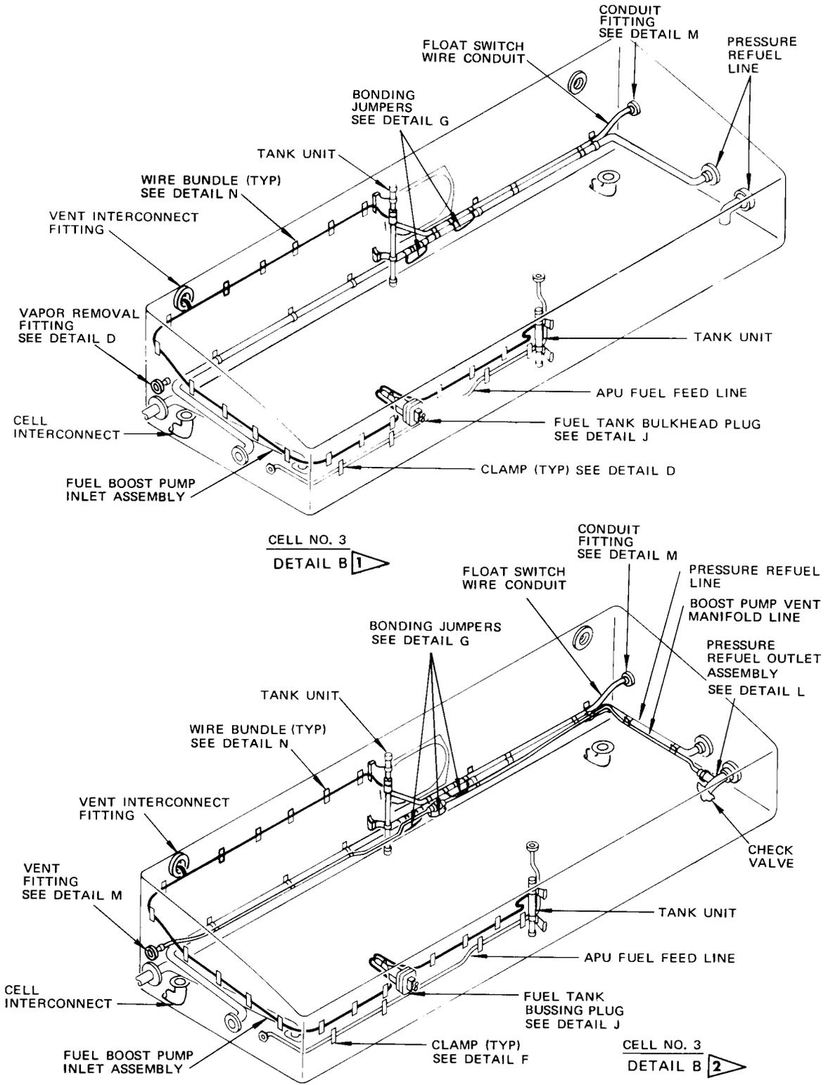
Fuel Cell Plumbing and Fitting Installation
