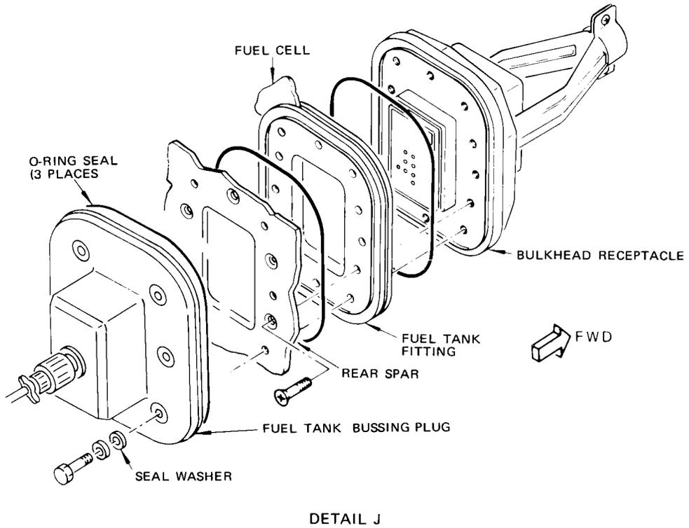
Fuel Cell Plumbing and Fitting Installation
