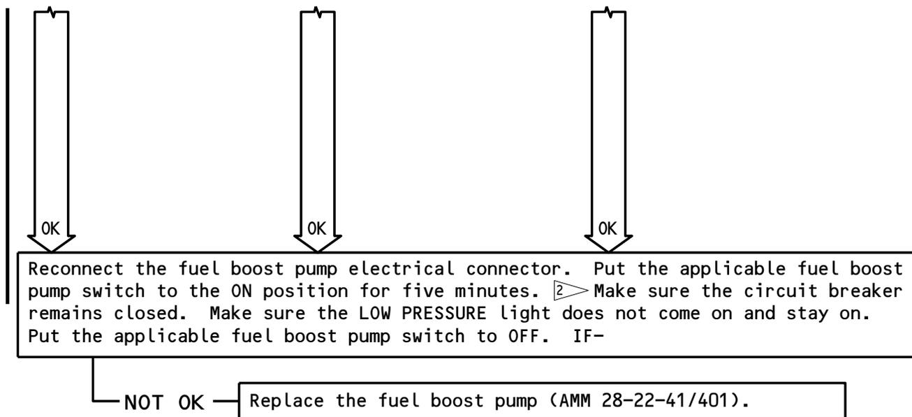
2 To operate any of the fuel boost pumps, you must be in the flight compartment to continuously monitor the fuel quantity and the low pressure indication in the fuel tank. Immediately put the applicable fuel boost pump switch(es) to OFF if the LOW PRESSURE light comes on and stays on.
