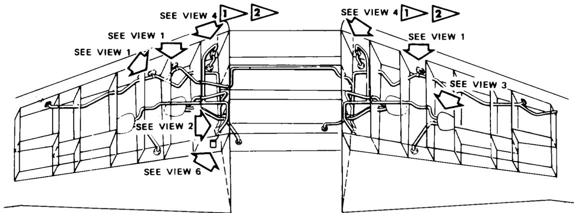
Engine Fuel Feed System Installation
