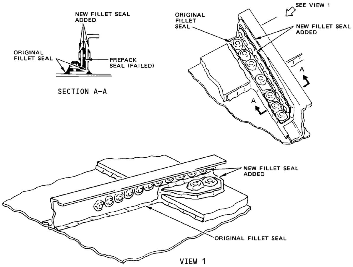
Raising the Seal Plane to Repair a Failed Prepack Seal
