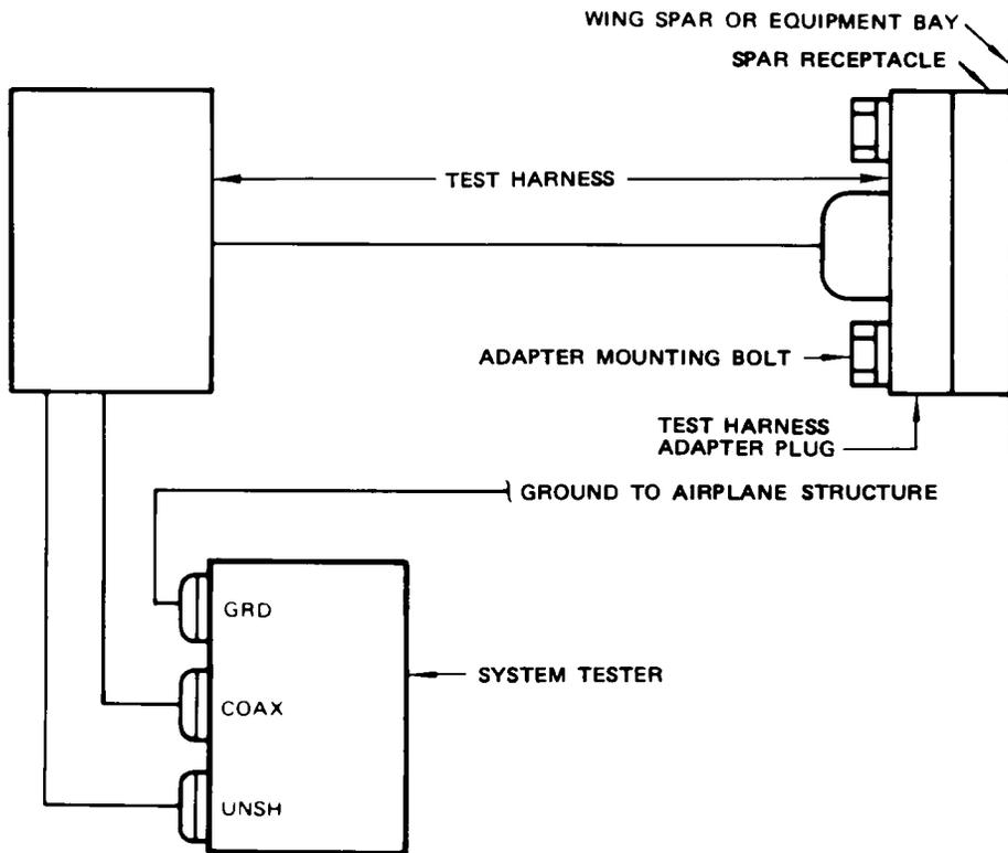
Tank Unit and Compensator Unit Test Connections
