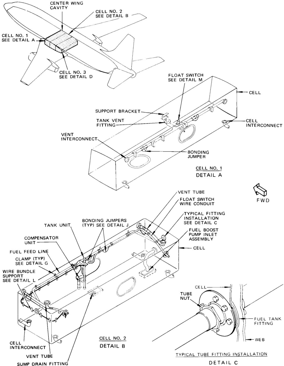
Fuel Cell Plumbing and Fitting Installation
