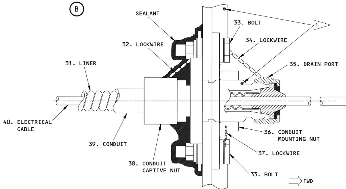
**1** RESISTANCE FROM THE FLOAT SWITCH CONDUIT TO THE FRONT SPAR MUST BE LESS THAN 0.010 OHM
