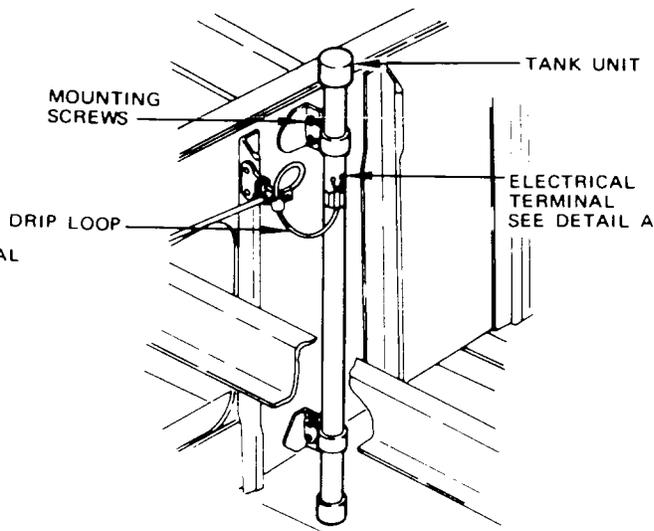
**Tank Unit and Compensator Unit Installation
