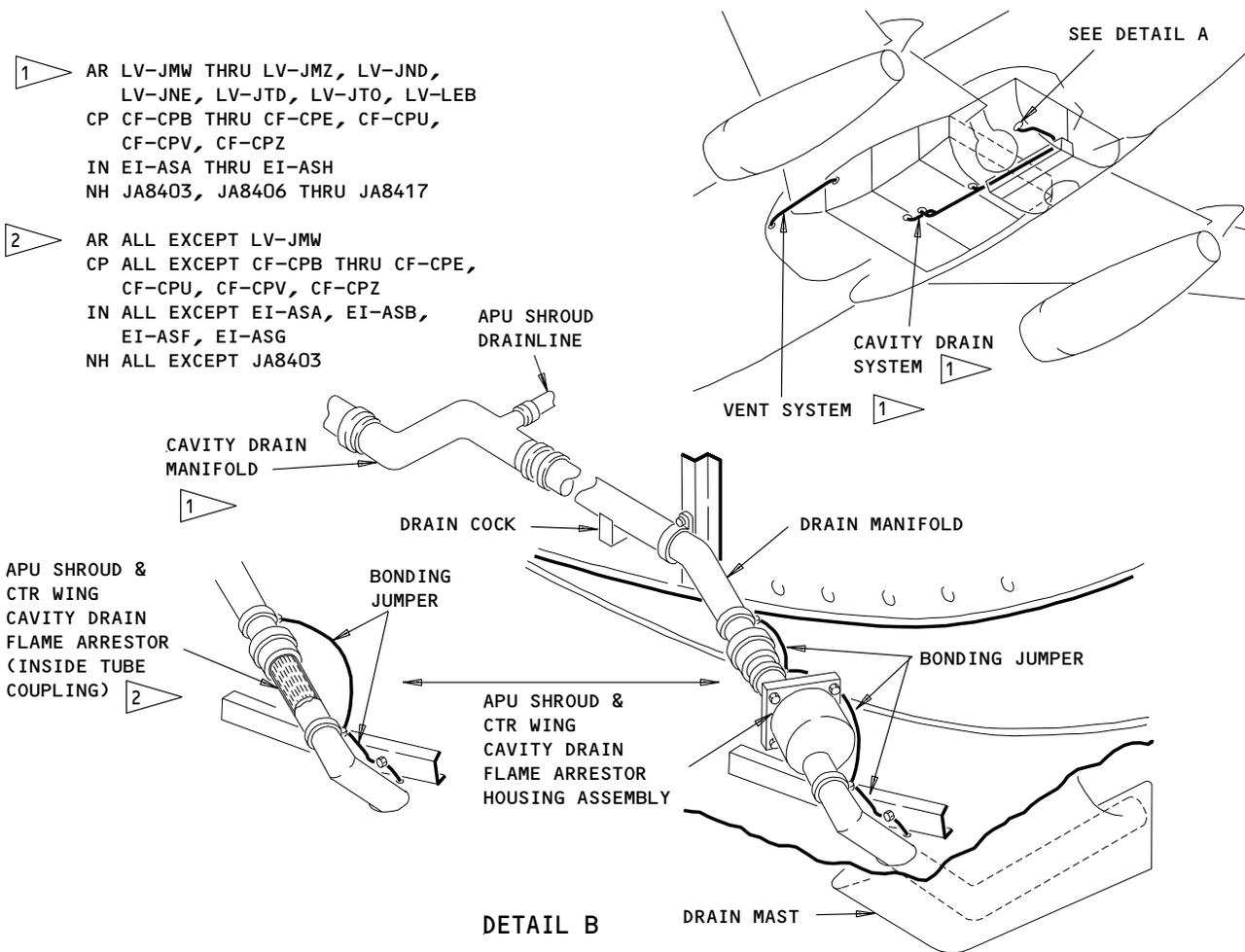
**Center Wing Cavity and APU Shroud Drain System
