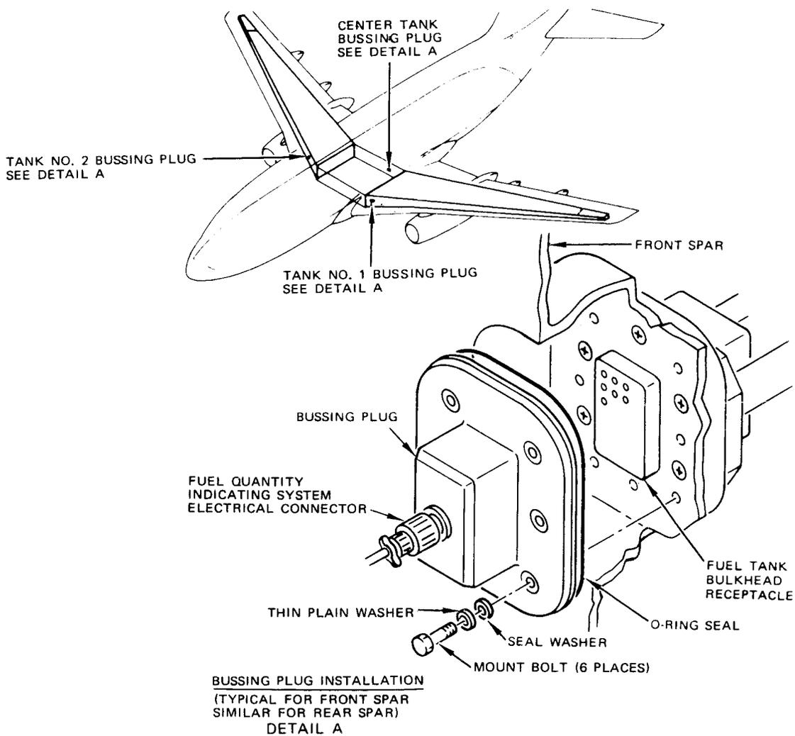
Tank Unit and Compensator Unit Bussing Plug Installation
