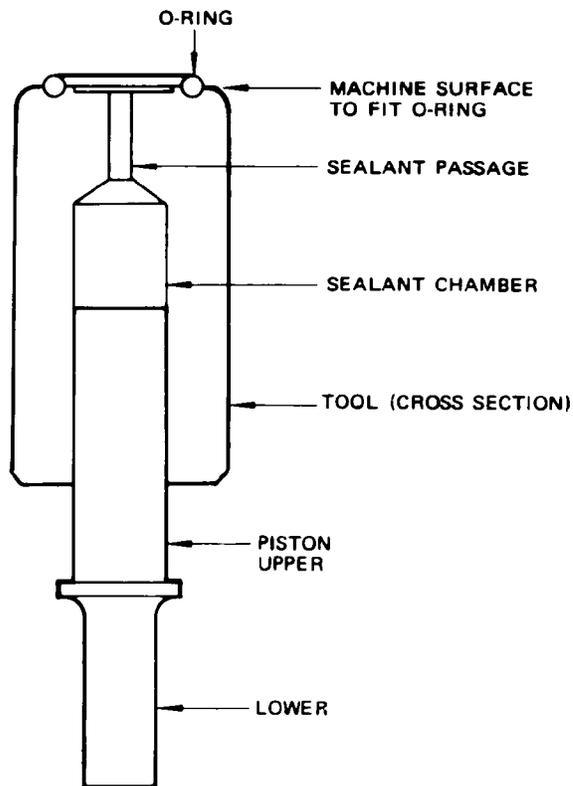
Fuel System Self-Sealing Rivets Temporary Repair Tool (F70230)
