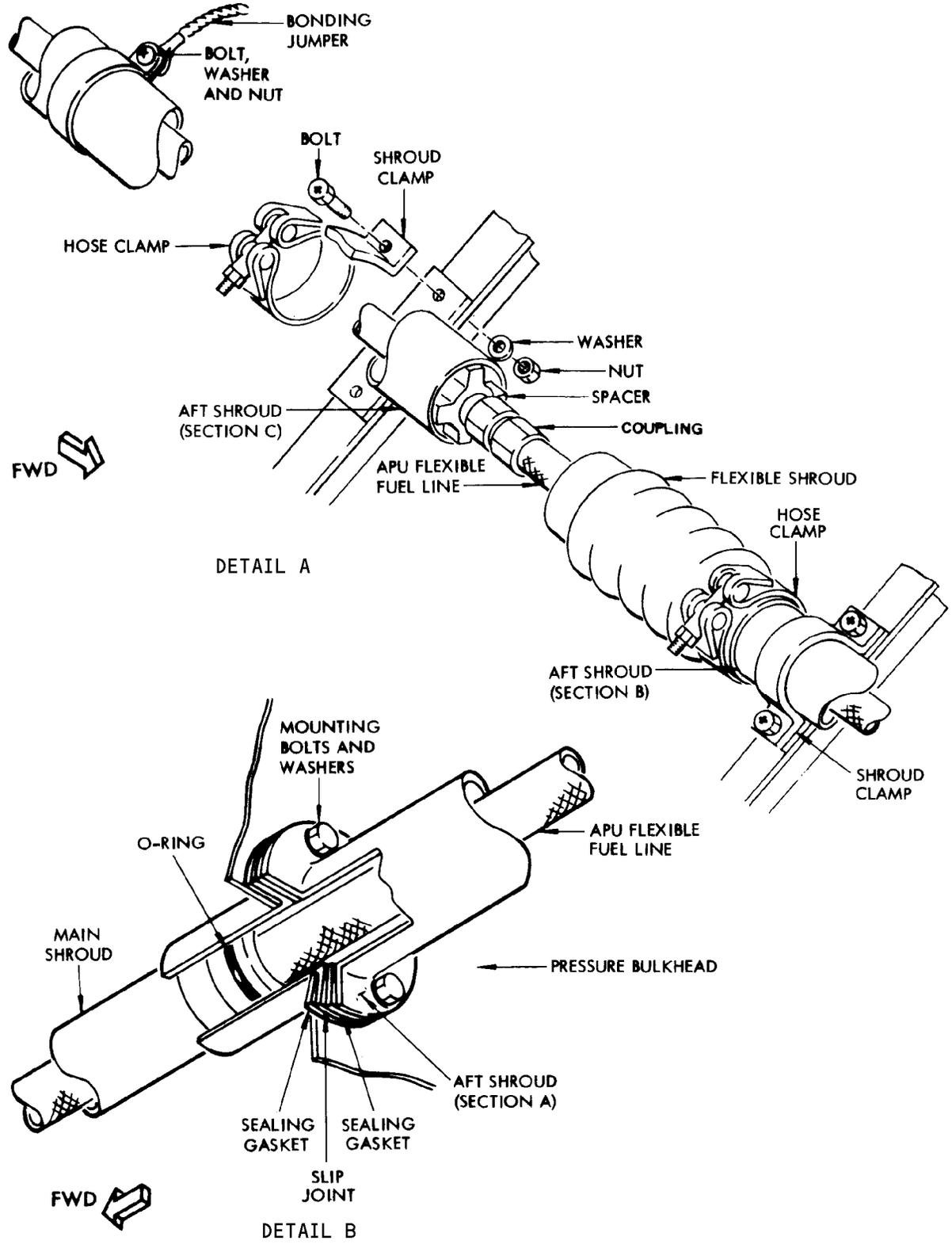
APU Fuel Feed Line Shroud Installation
