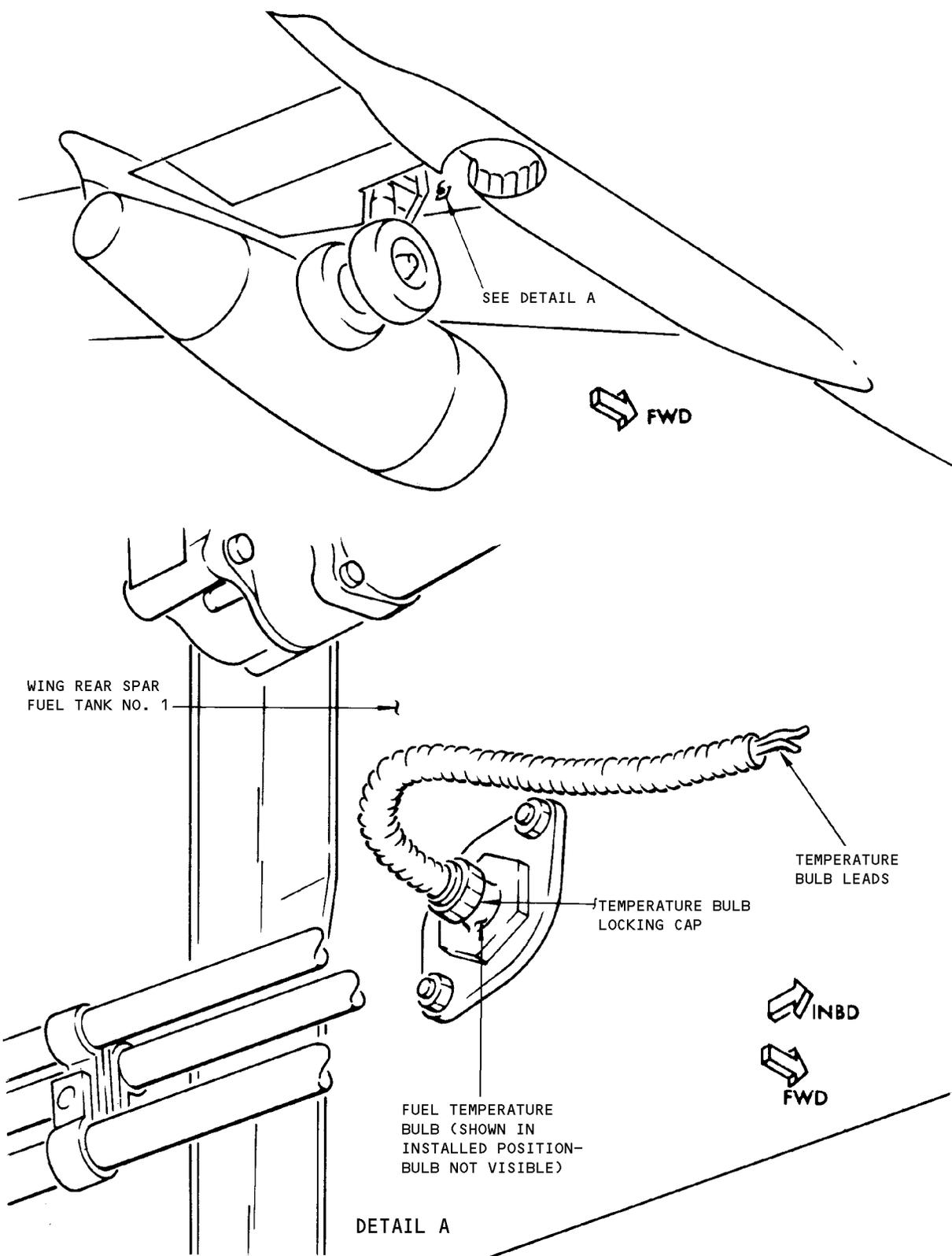
Fuel Temperature Bulb Installation
