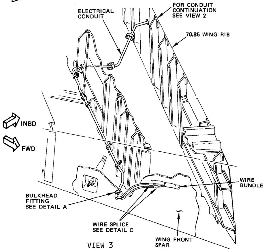
Fueling Float Switch Installation (Type I)
