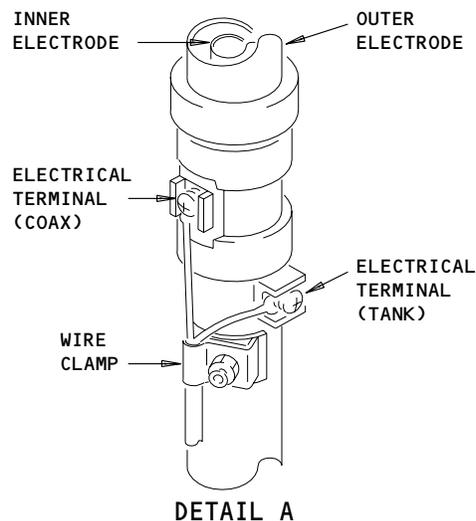
Tank Unit and Compensator Unit Installation
