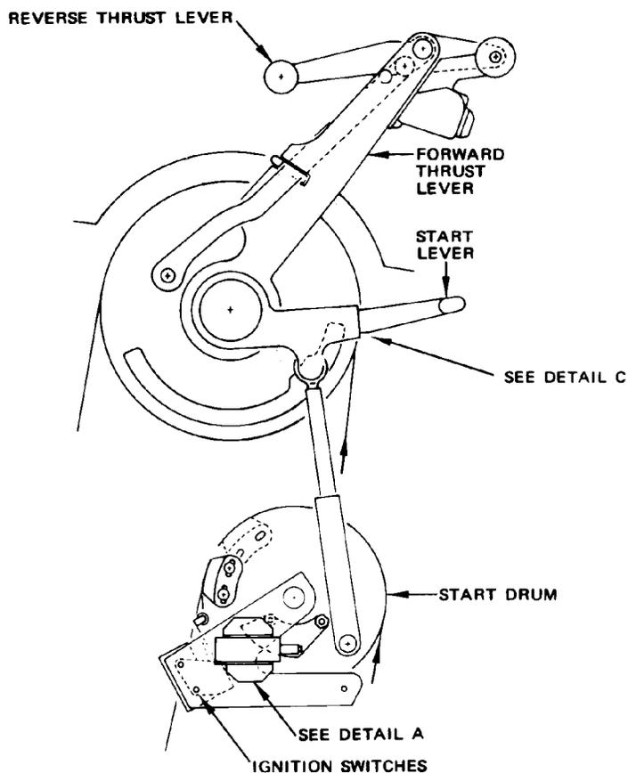
Engine Fuel Shutoff Valve Switch Adjustment
