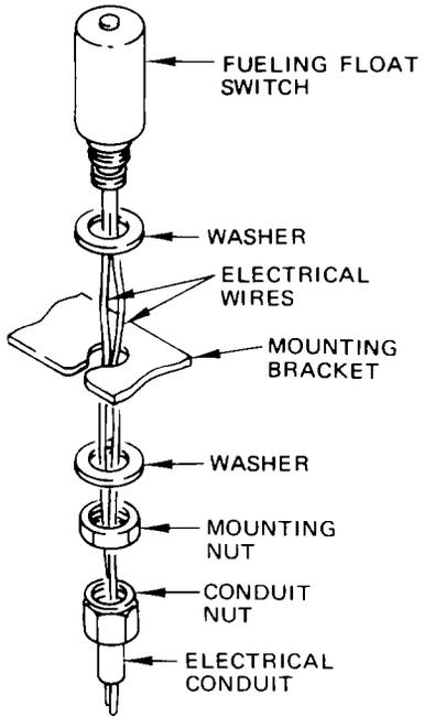
FUELING FLOAT SWITCH INSTALLATION (TYPICAL)
