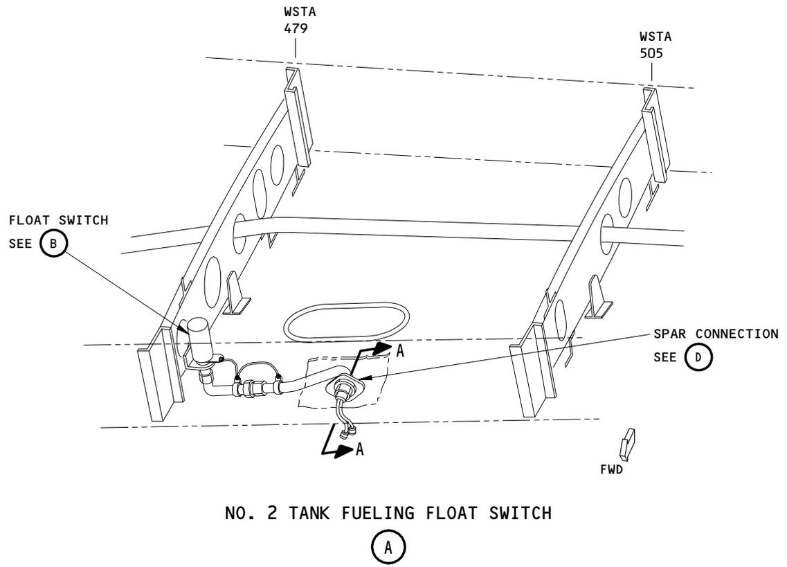
Main Tank Float Switch and Conduit Installation (Type II)
