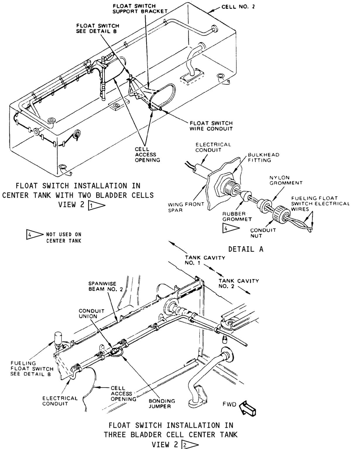
Fueling Float Switch Installation (Type I)
