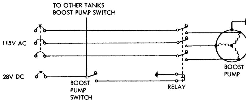
TYPICAL CIRCUIT FOR ONE BOOST PUMP IN A GIVEN TANK. OTHER BOOST PUMP CIRCUIT SAME BUT WITH SEPARATE SOURCE OF POWER AS SHOWN IN TABLE BELOW
