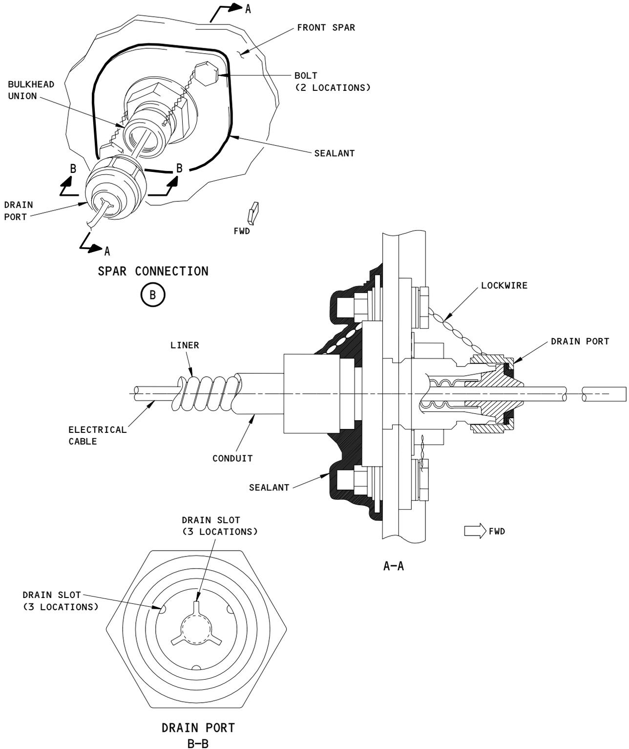
Center Tank Float Switch (Type II) Drain Port
