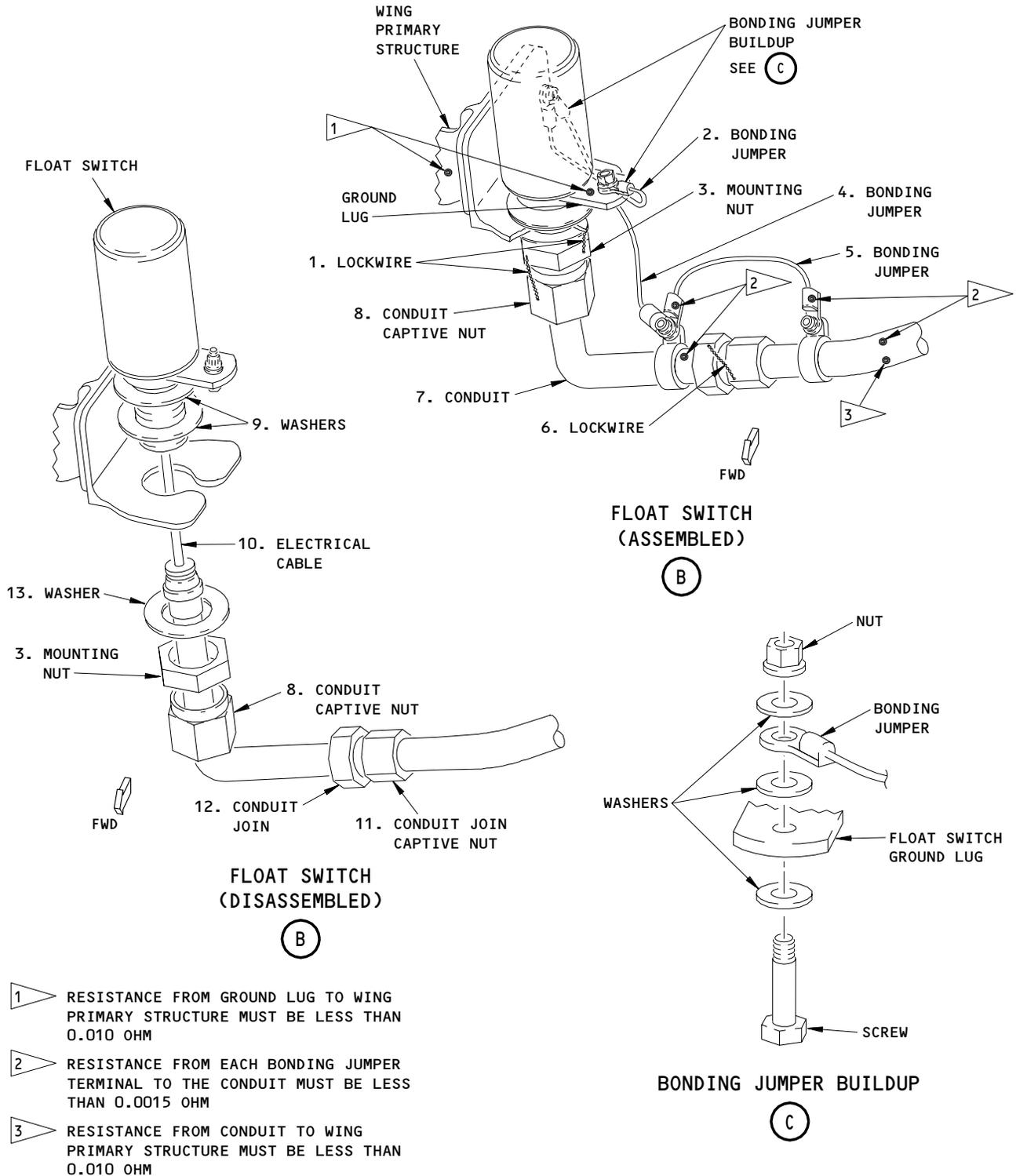
Main Tank Float Switch and Conduit Installation (Type II)
