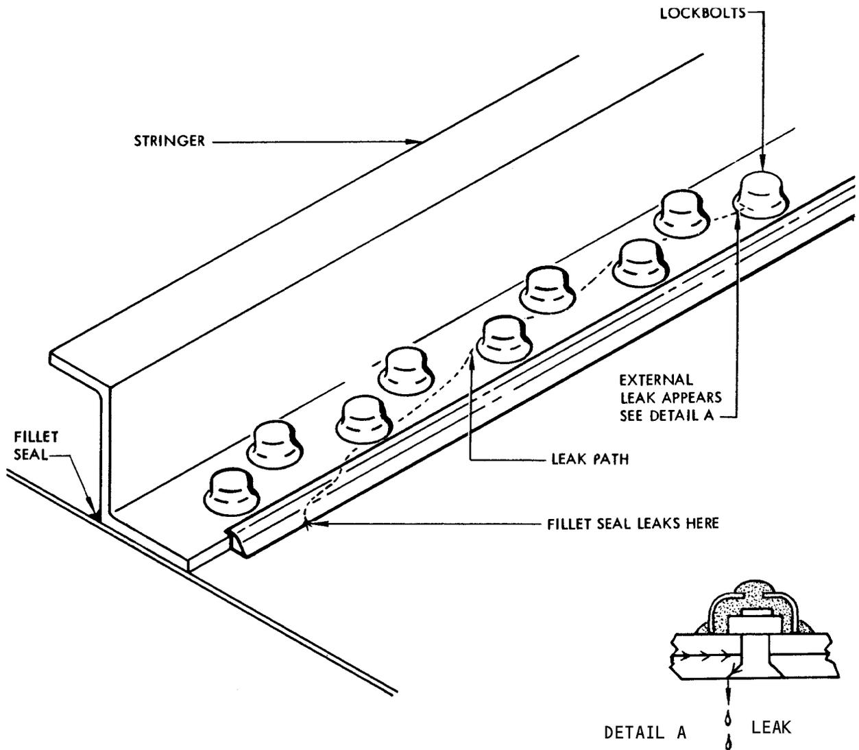
Typical Fillet Seal Leak
