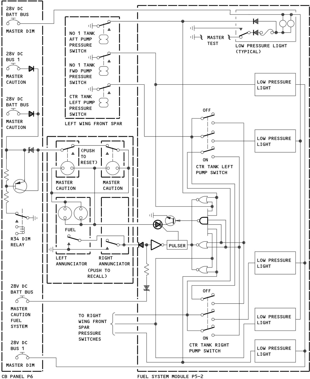
**Boost Pump Low Pressure Indicating Light Circuit**
