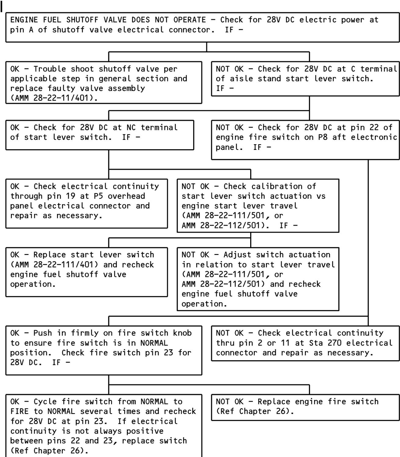
Engine Fuel Shutoff Valve Does Not Operate
