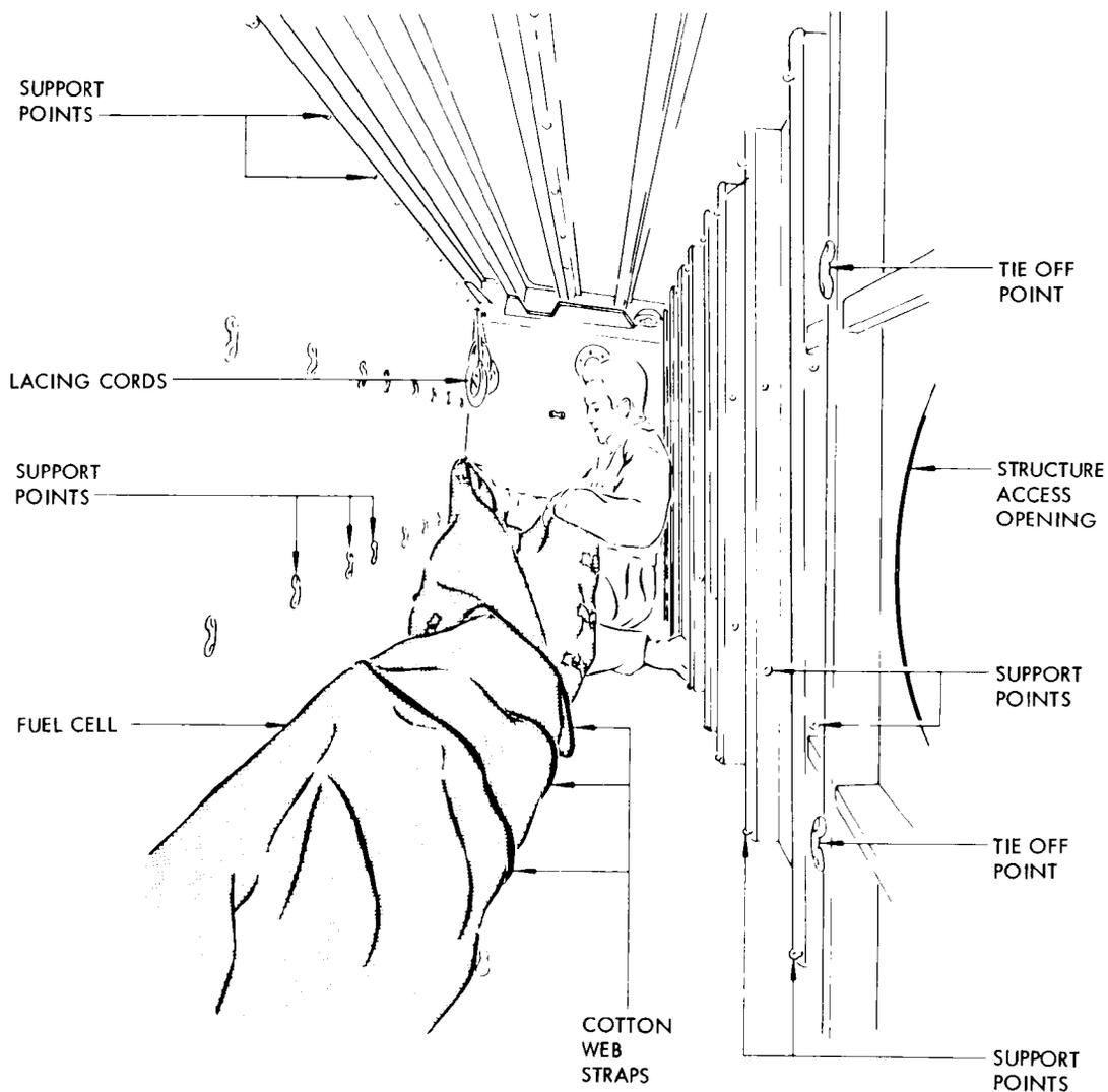
Fuel Cell Unfolding and Lacing
