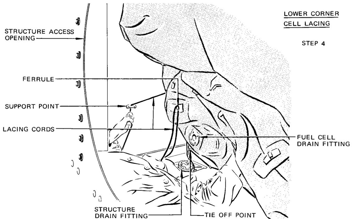
Fuel Cell Unfolding and Lacing
