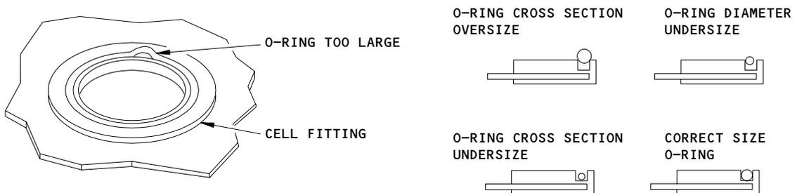
O-Ring Groove Preparation and Fit
