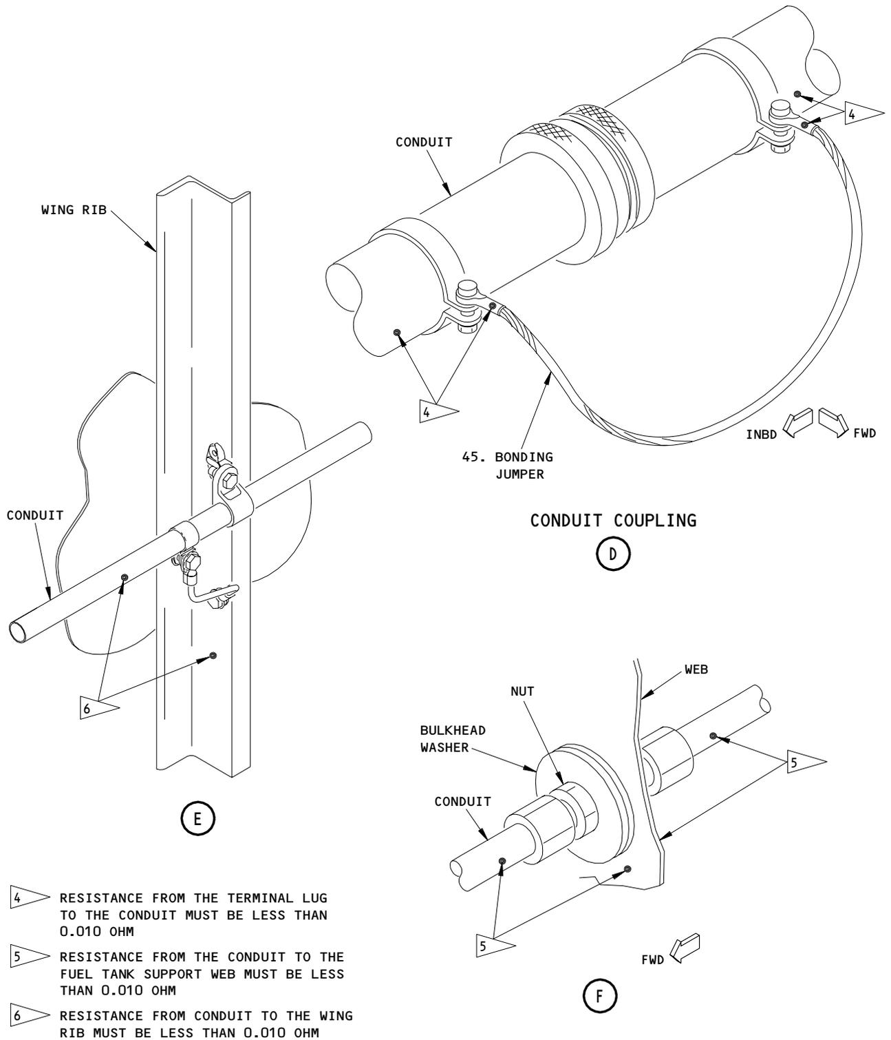
Center Tank Float Switch Installation (Type II)
