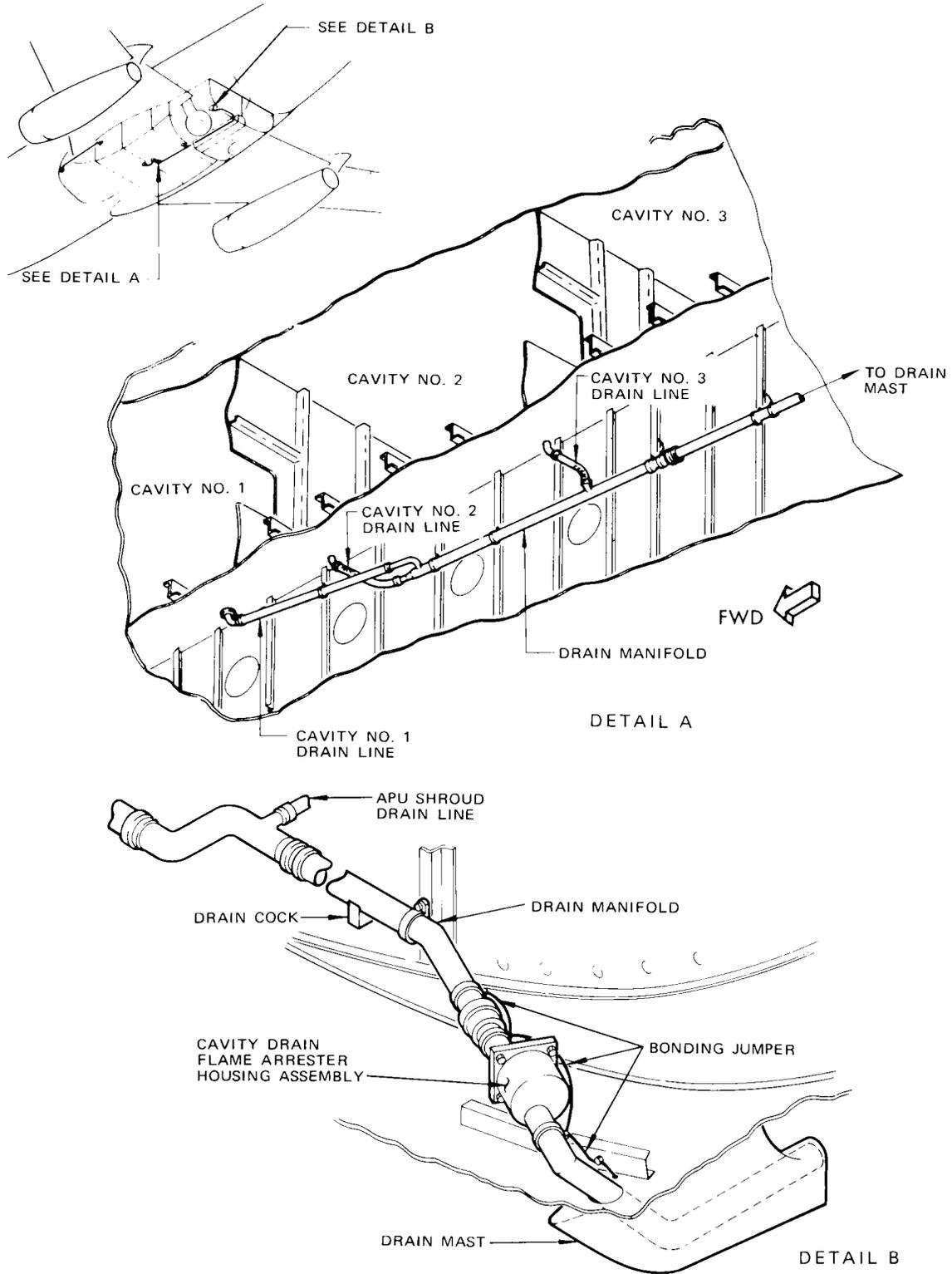
Center Wing Cavity Drain System
