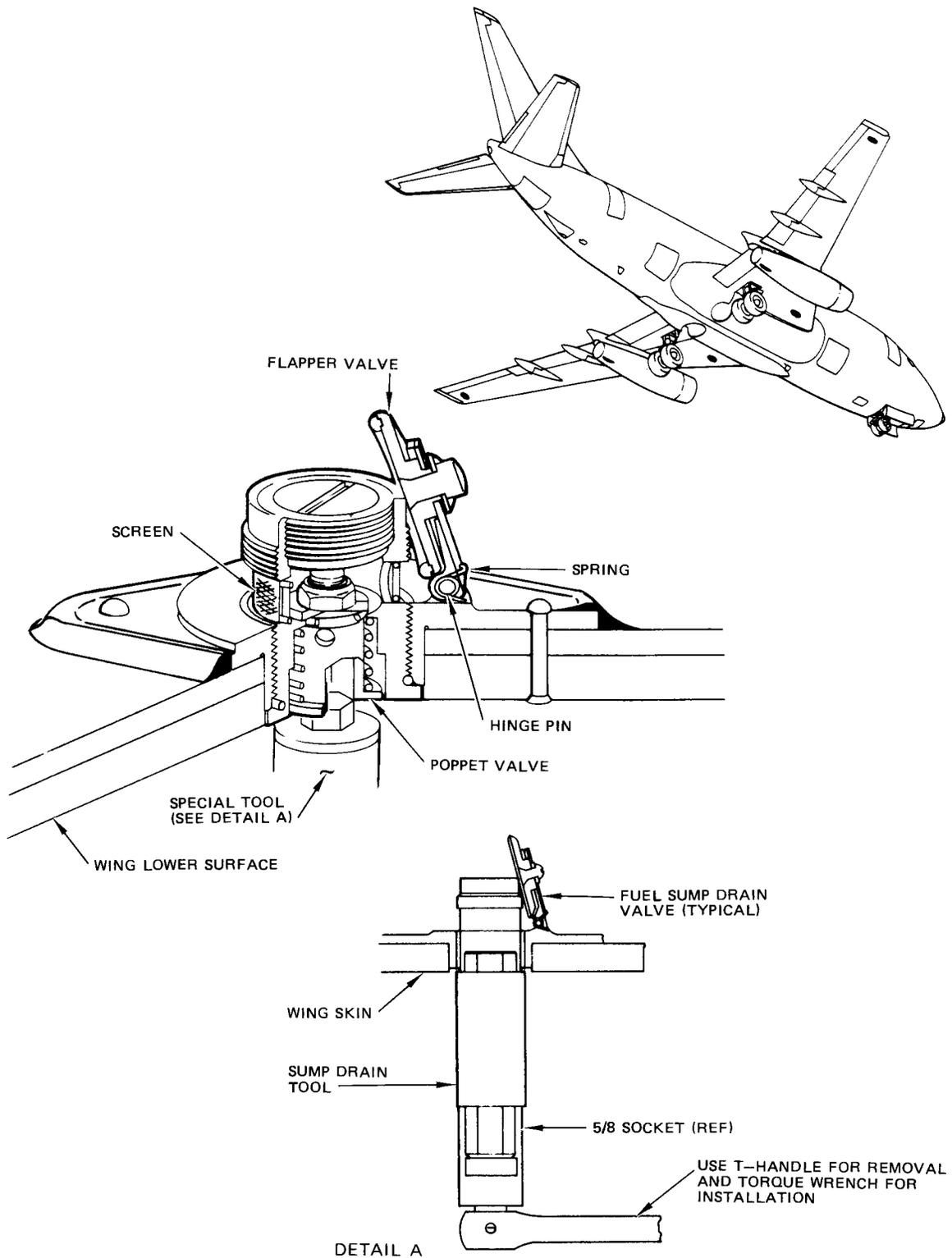
Fuel Sump Drain Valve Installation (Typical)
