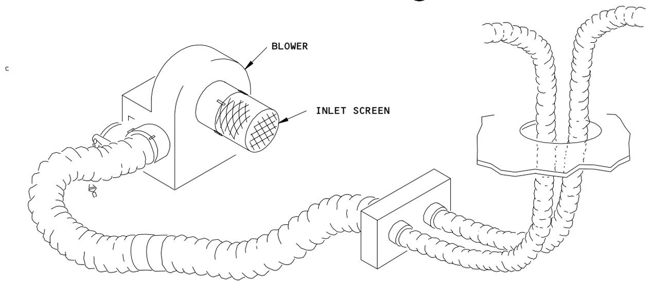
**EXAMPLE CONFIGURATION FOR VENTILATION EQUIPMENT (MODEL BOE-501)**
