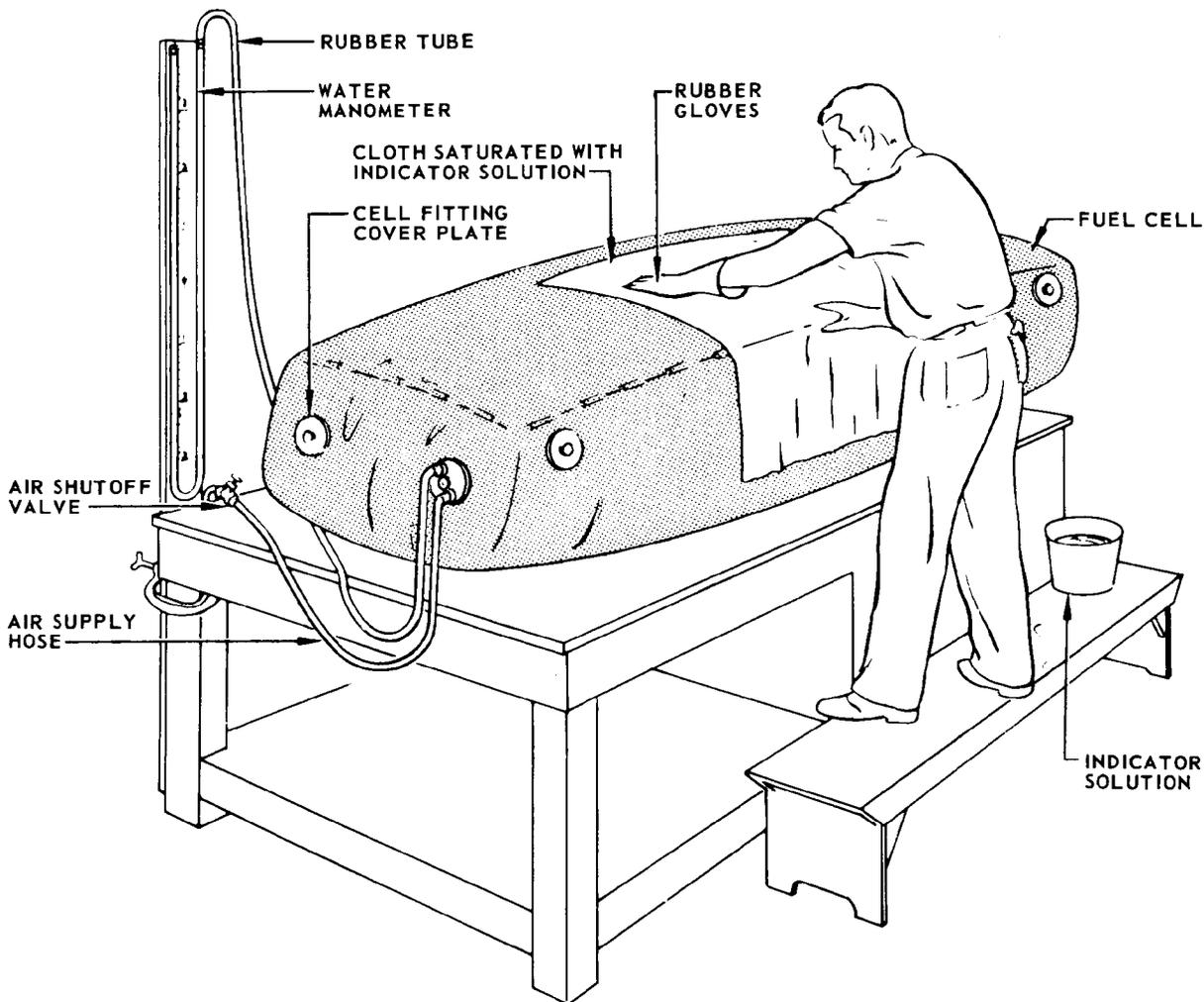
Fuel Cell Chemical Leak Test
