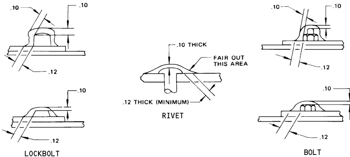
Dimensions of Fasteners Fillet Seals (Inches)
