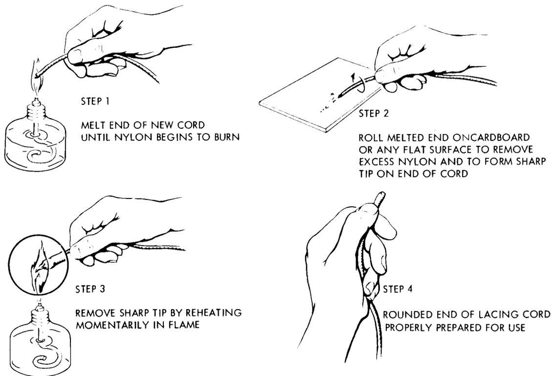
Preparing End of Fuel Cell Lacing Cord for Installation
