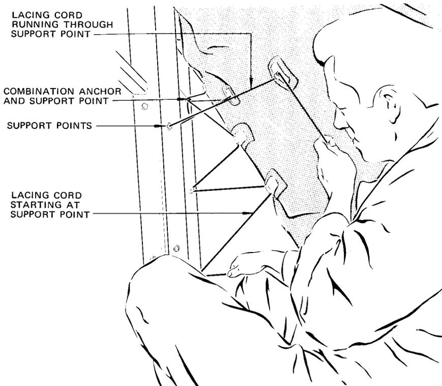
COMBINATION ANCHOR AND SUPPORT POINT LACING
