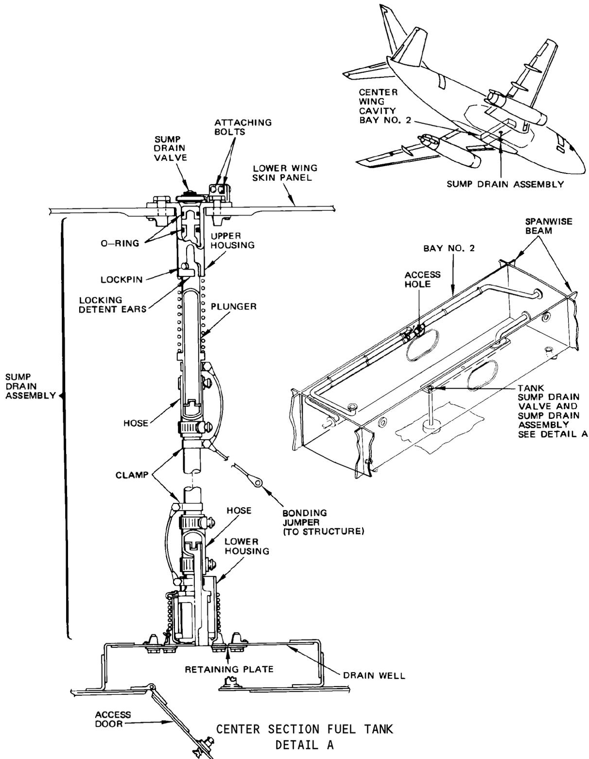
Center Tank Sump Drain Assembly and Drain Valve Installation
