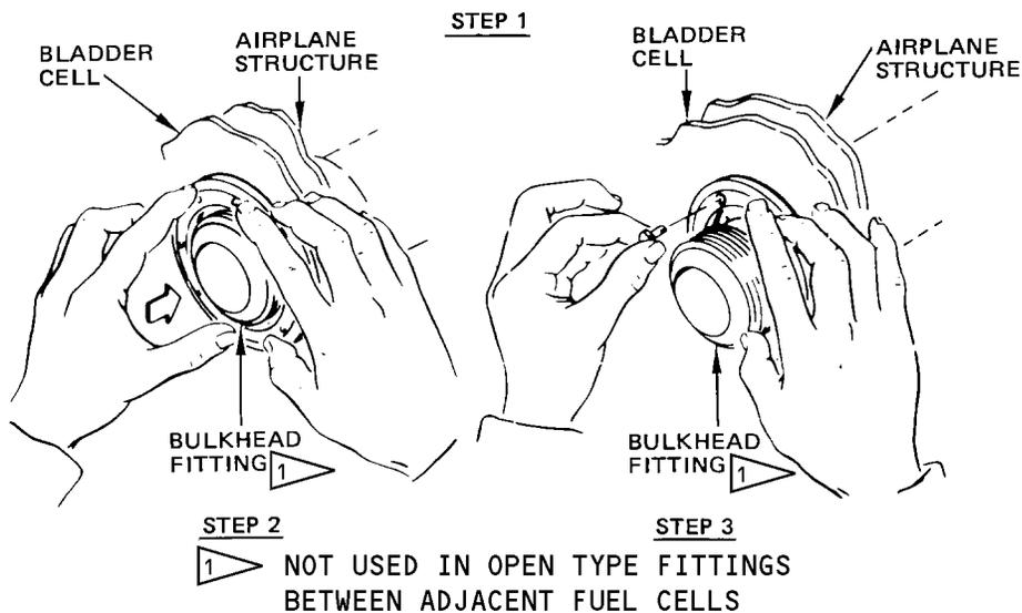
Fuel Cell Fitting Installation
