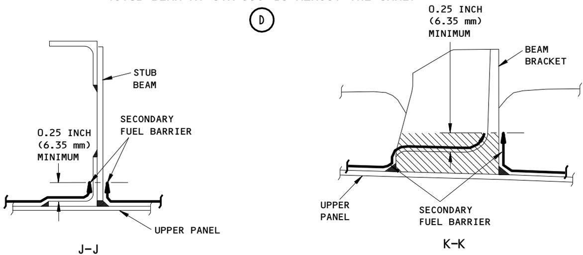
**Secondary Fuel Barrier Sealant Repair**
