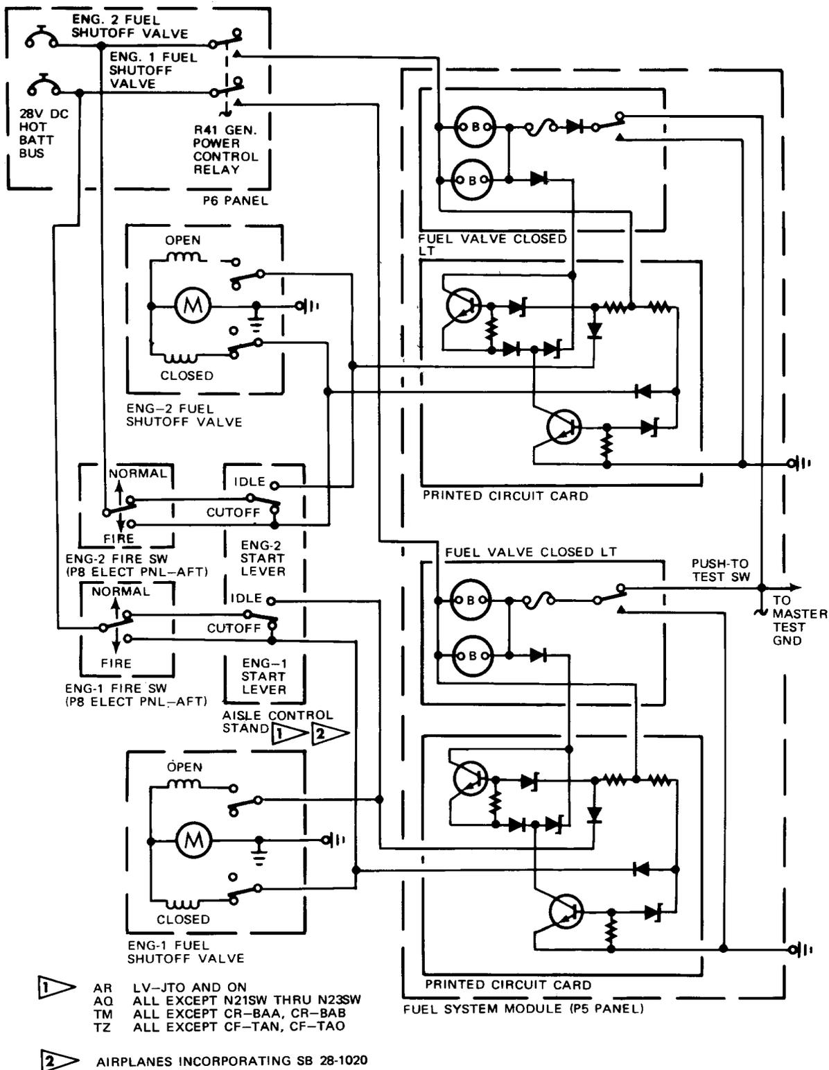
Engine Fuel Shutoff Valve Circuit
