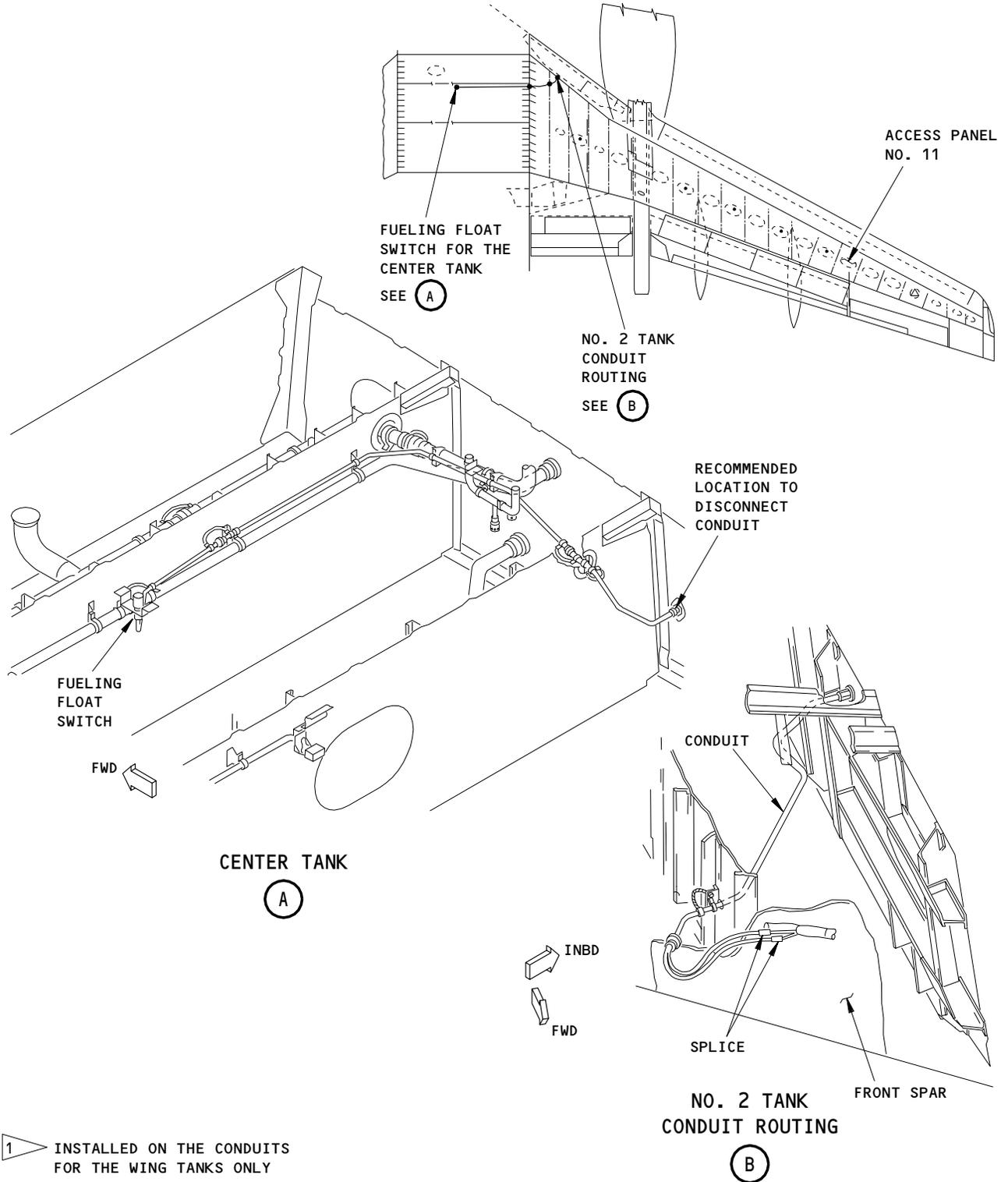
Fueling Float Switch and Conduit Inspection
