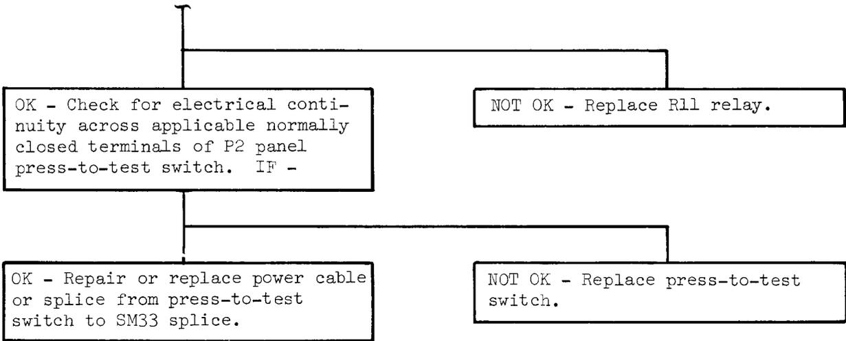
NOTE: Refer to Wiring Diagram Manual (WDM) for wiring details.
