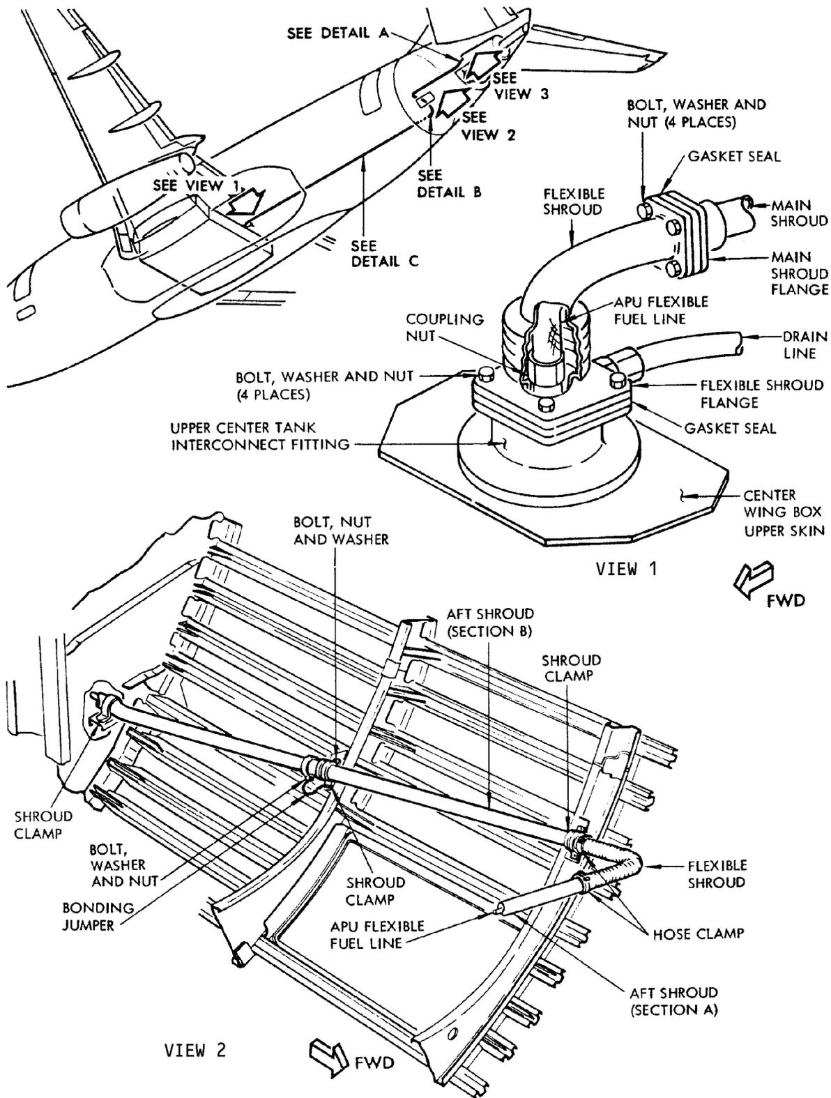
APU Fuel Feed Line Shroud Installation
