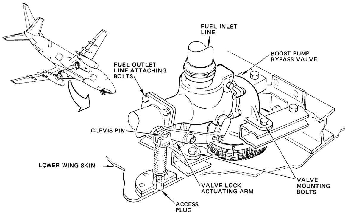
Boost Pump Bypass Valve Installation (Typical)
