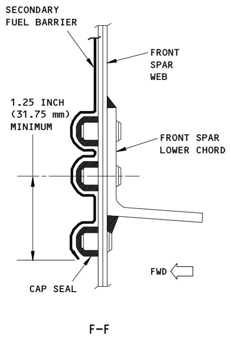
Secondary Fuel Barrier Sealant Repair
