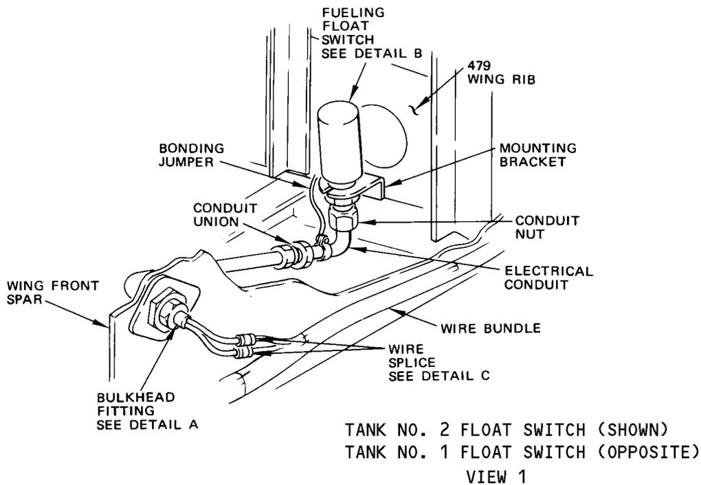
Fueling Float Switch Installation (Type I)
