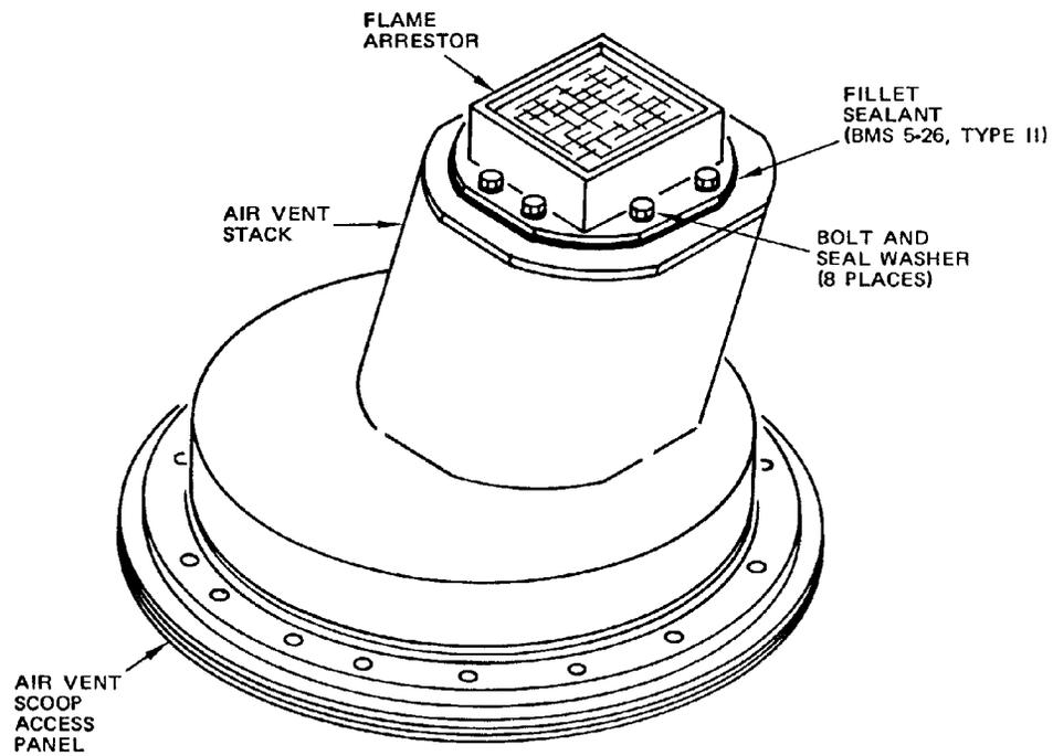
Air Vent Scoop Flame Arrestor Installation
