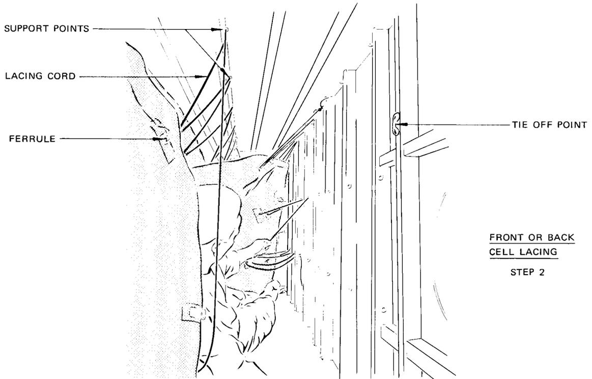
Fuel Cell Unfolding and Lacing
