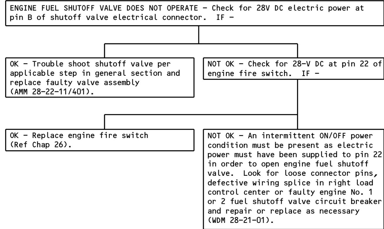
Engine Fuel Shutoff Valve Does Not Operate
