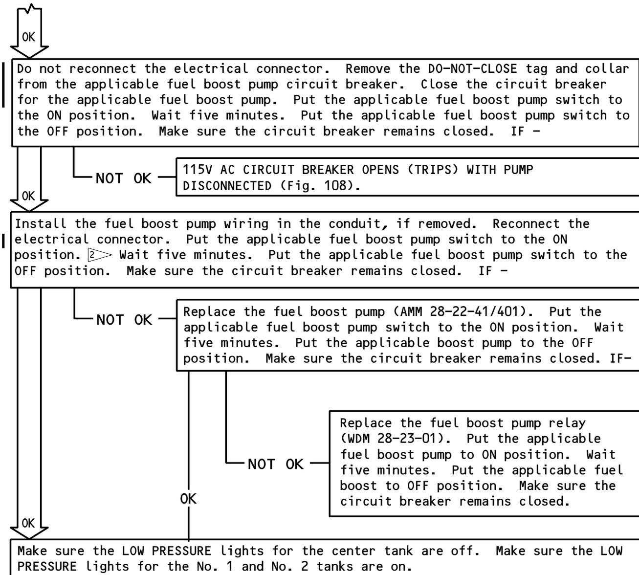
2 To operate any of the fuel boost pumps, you must be in the flight compartment to continuously monitor the fuel quantity and the low pressure indication in the fuel tank. Immediately put the applicable fuel boost pump switch(es) to OFF if the LOW PRESSURE light comes on and stays on.
