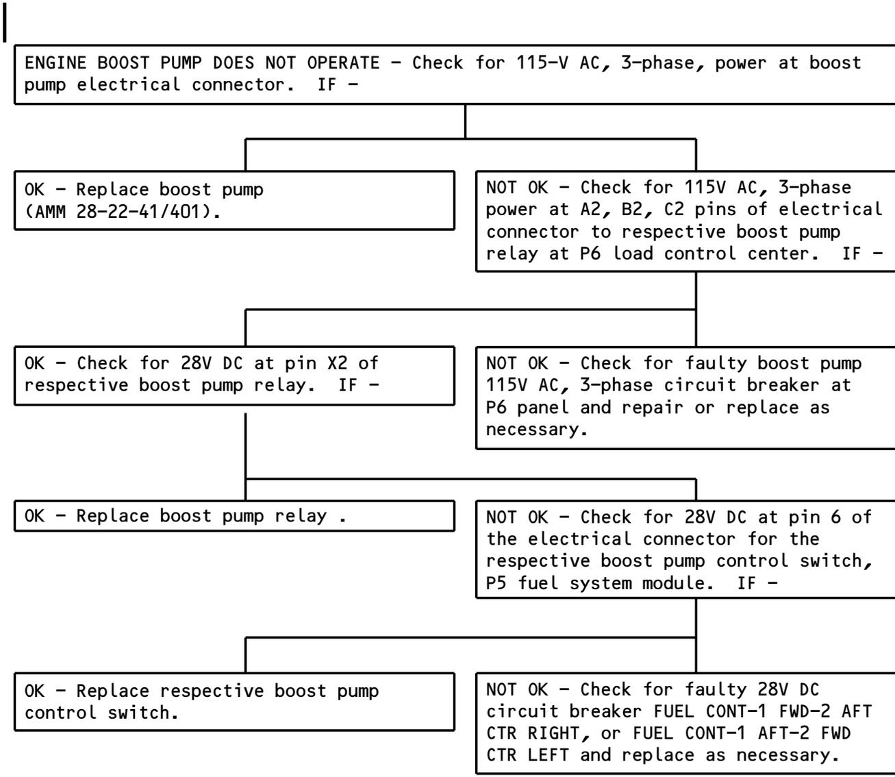
Engine Boost Pump Does Not Operate
