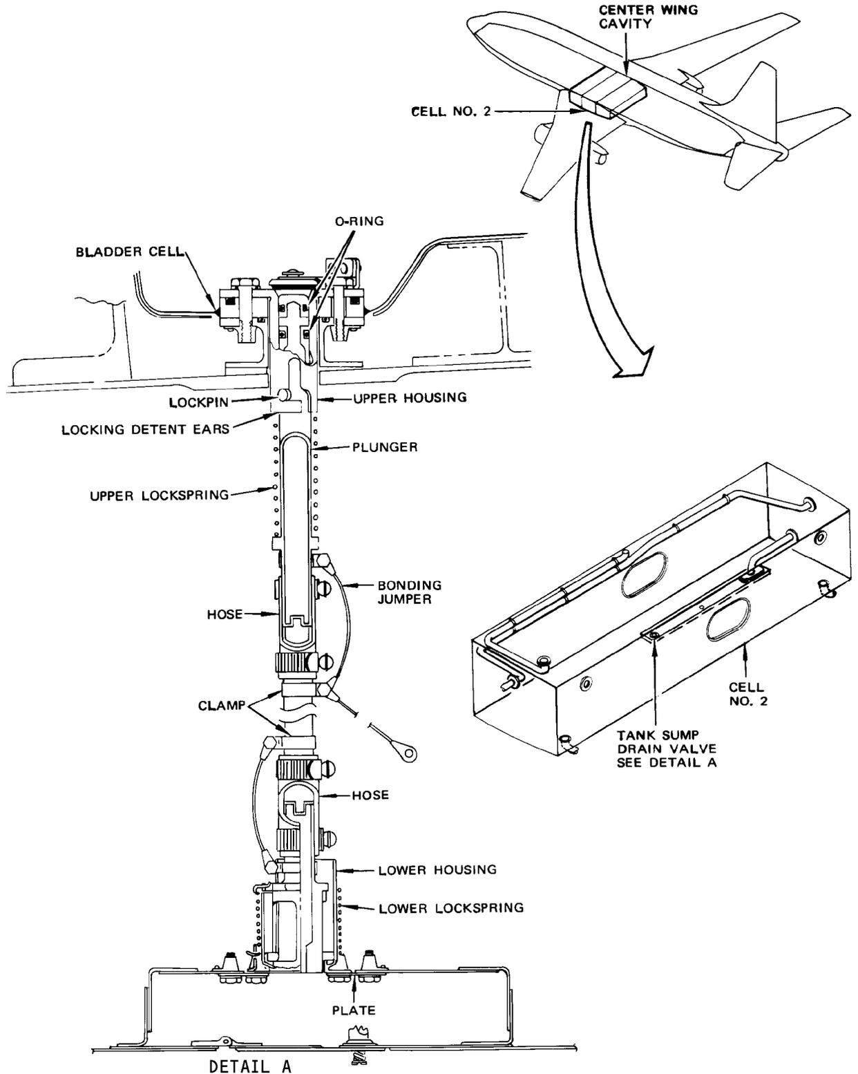
Center Tank Sump Drain Valve Installation
