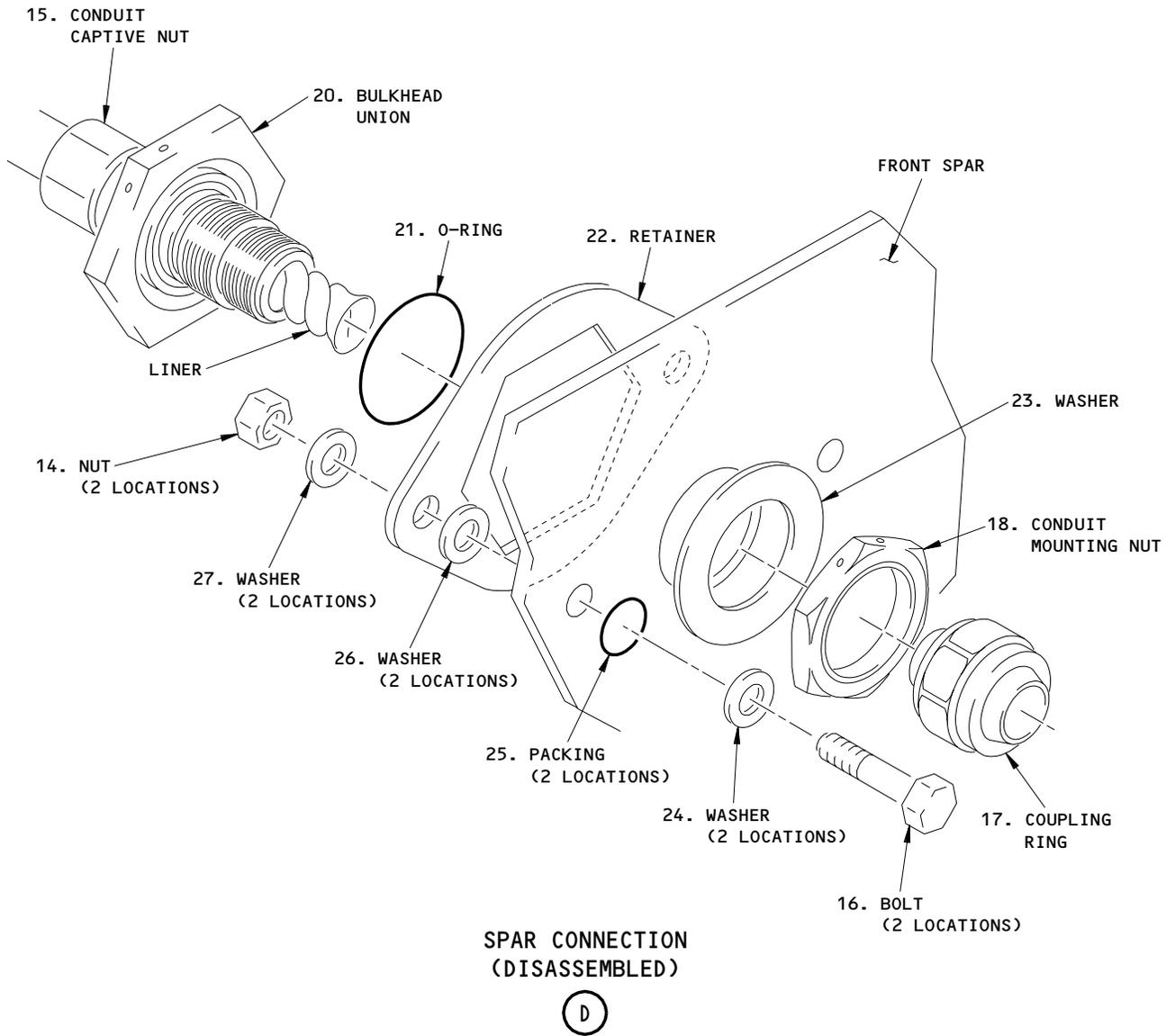
Main Tank Float Switch and Conduit Installation (Type II)
