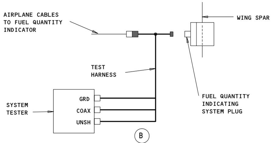
Fuel Quantity Indicating System Test Connections
