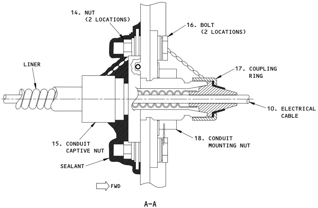
**Main Tank Float Switch and Conduit Installation (Type II)
