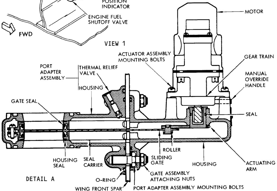
Engine Fuel Shutoff Valve Installation
