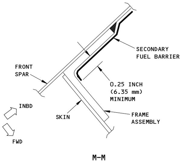
Secondary Fuel Barrier Sealant Repair
