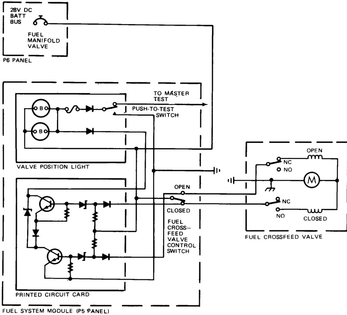
Fuel Crossfeed Valve Circuit
