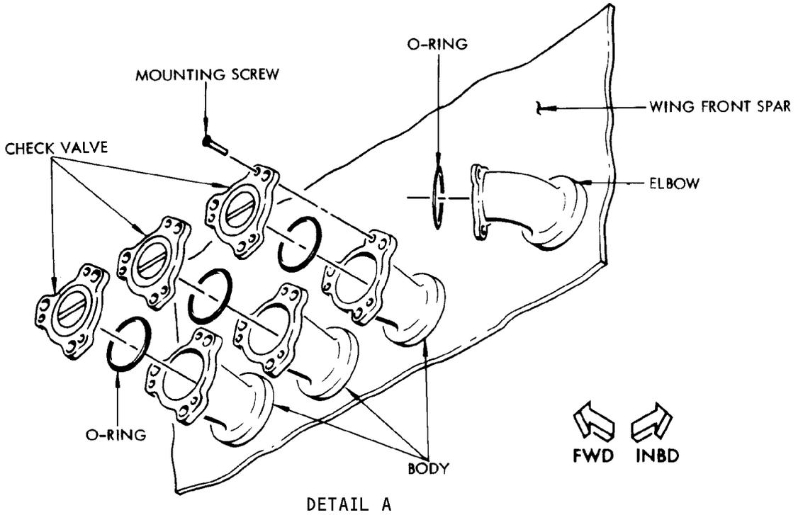
Fueling Check Valve Installation
