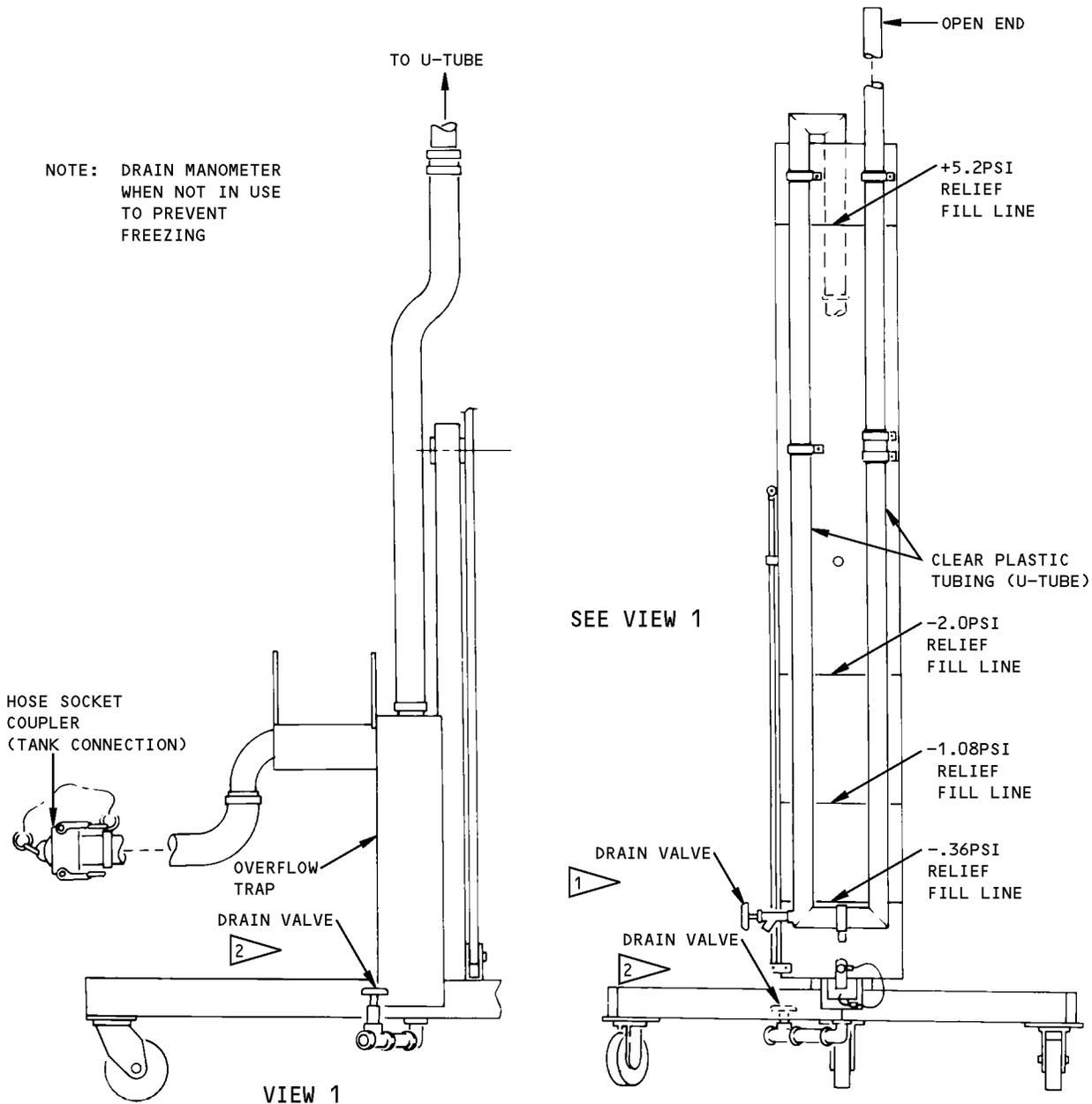
PREFERRED SAFETY TO ADJUST FILL LEVEL AND TO DRAIN TUBING
