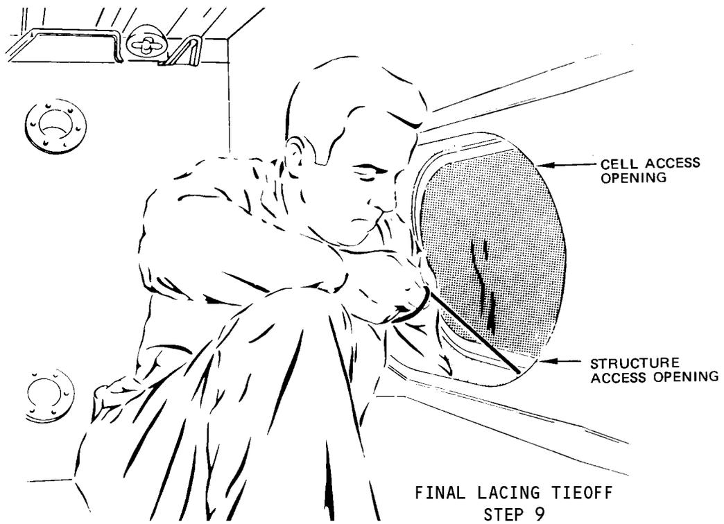
Fuel Cell Unfolding and Lacing
