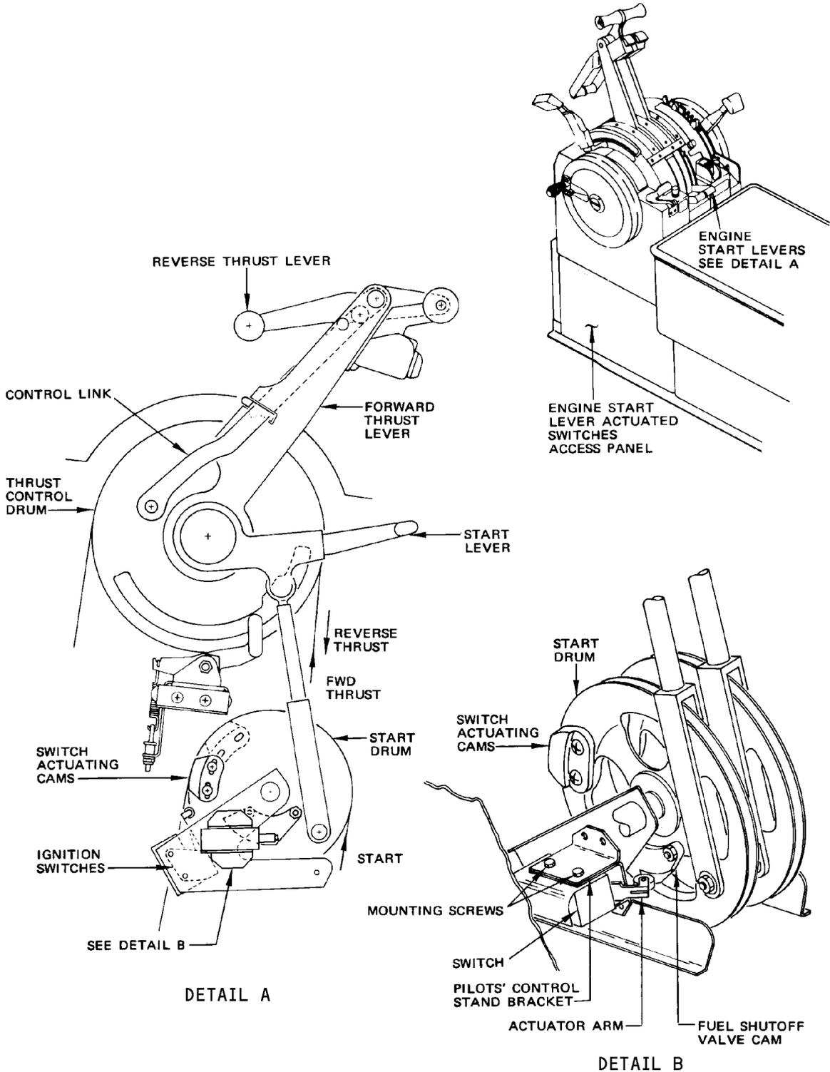
Engine Fuel Shutoff Valve Switch Installation
