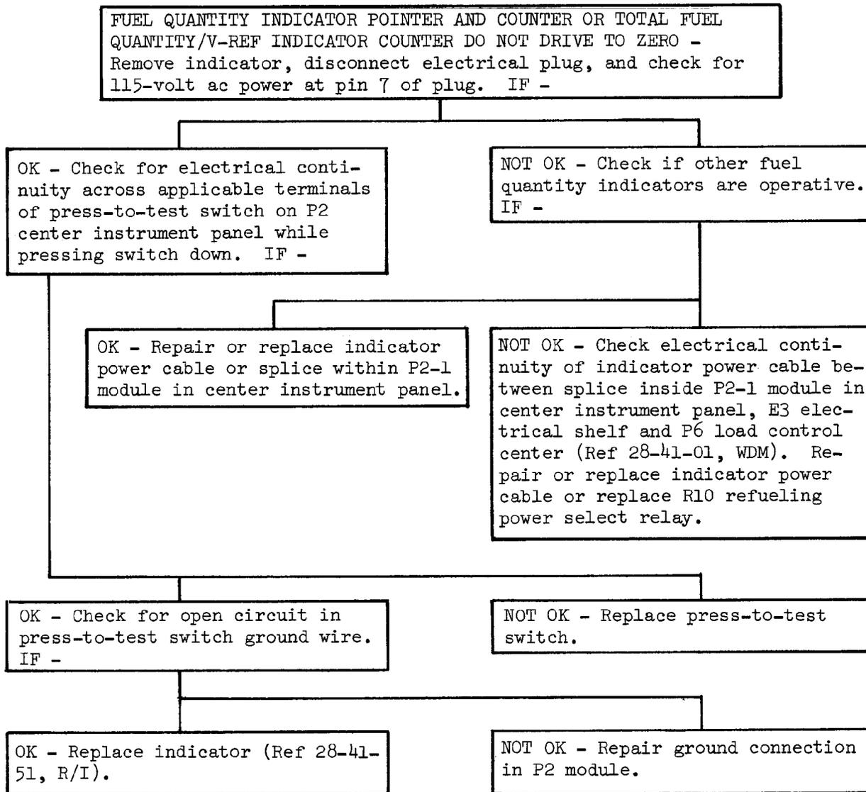
NOTE; Refer to Wiring Diagram Manual (WDM) for wiring details.
