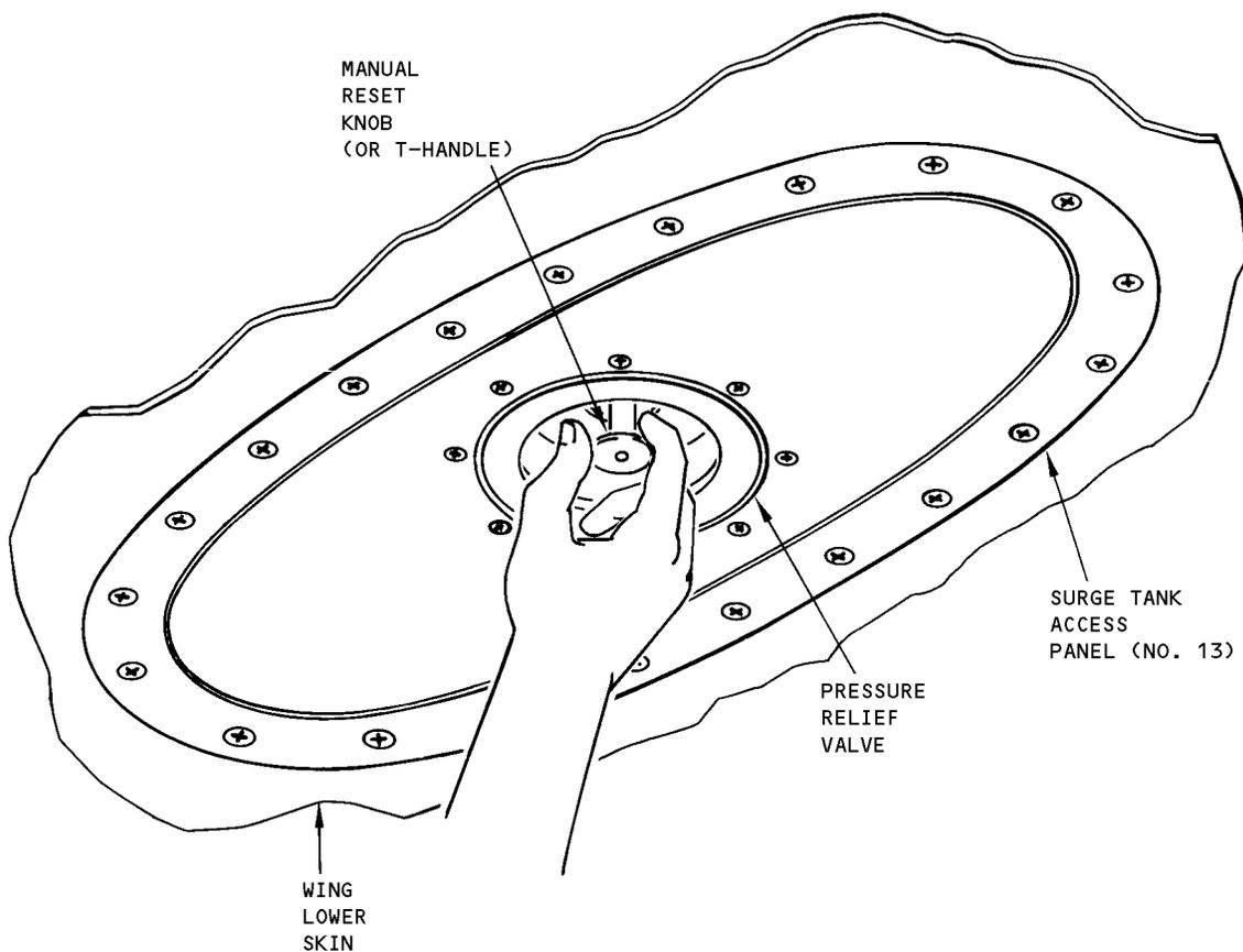
Surge Tank Flame Arrestor Pressure Relief Valve Manual Reset
