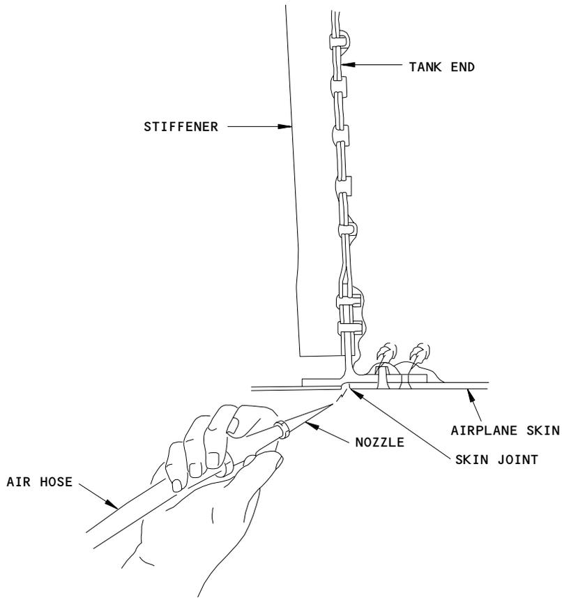
Leak Detection Air Hose and Bubble Method
