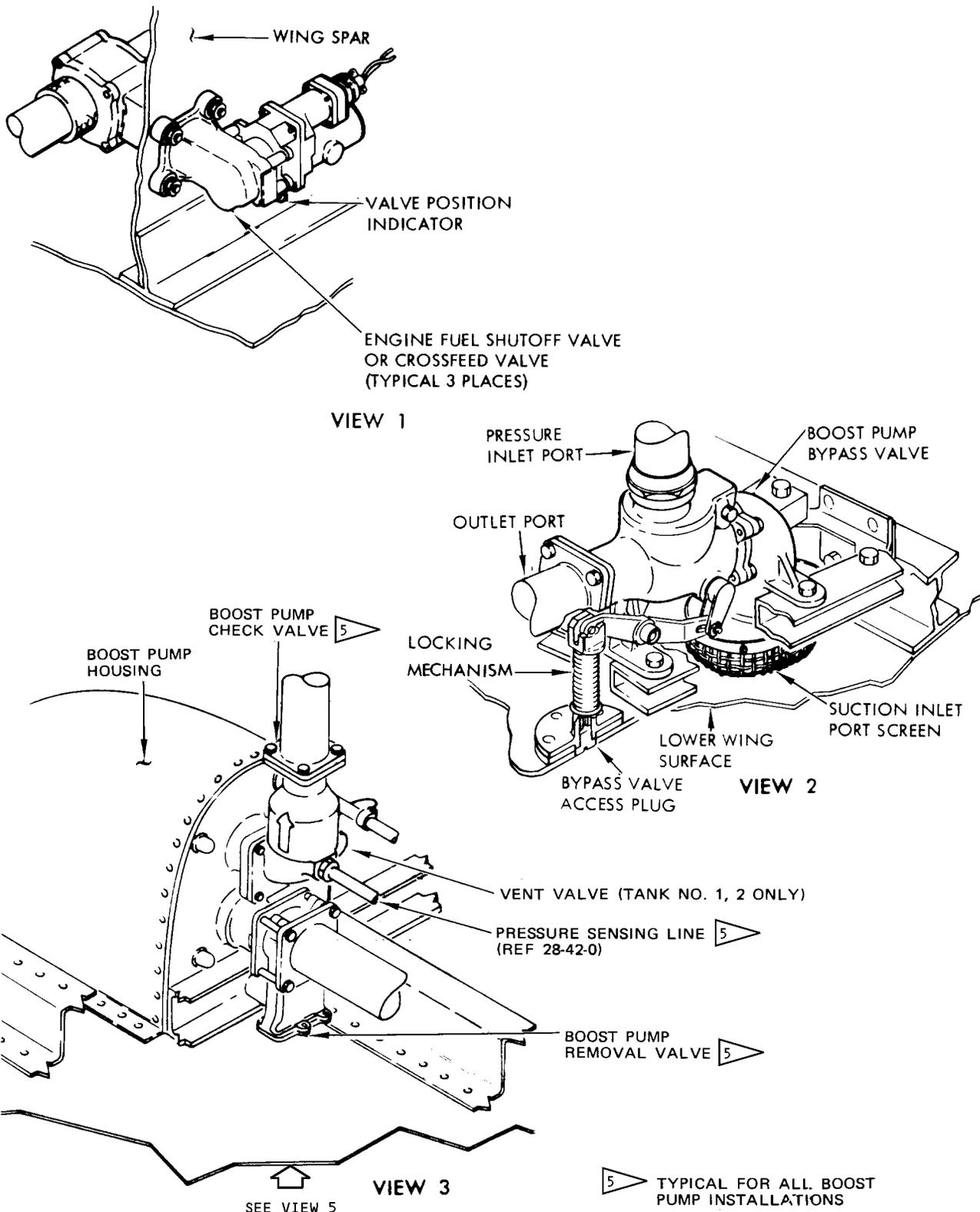
Engine Fuel Feed System Component Location
