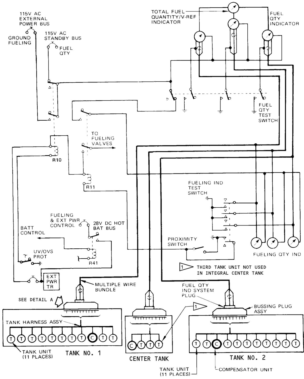
Fuel Quantity Indicating System Schematic
