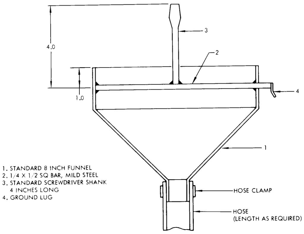
Center Wing Sump Drain Funnel Assembly
