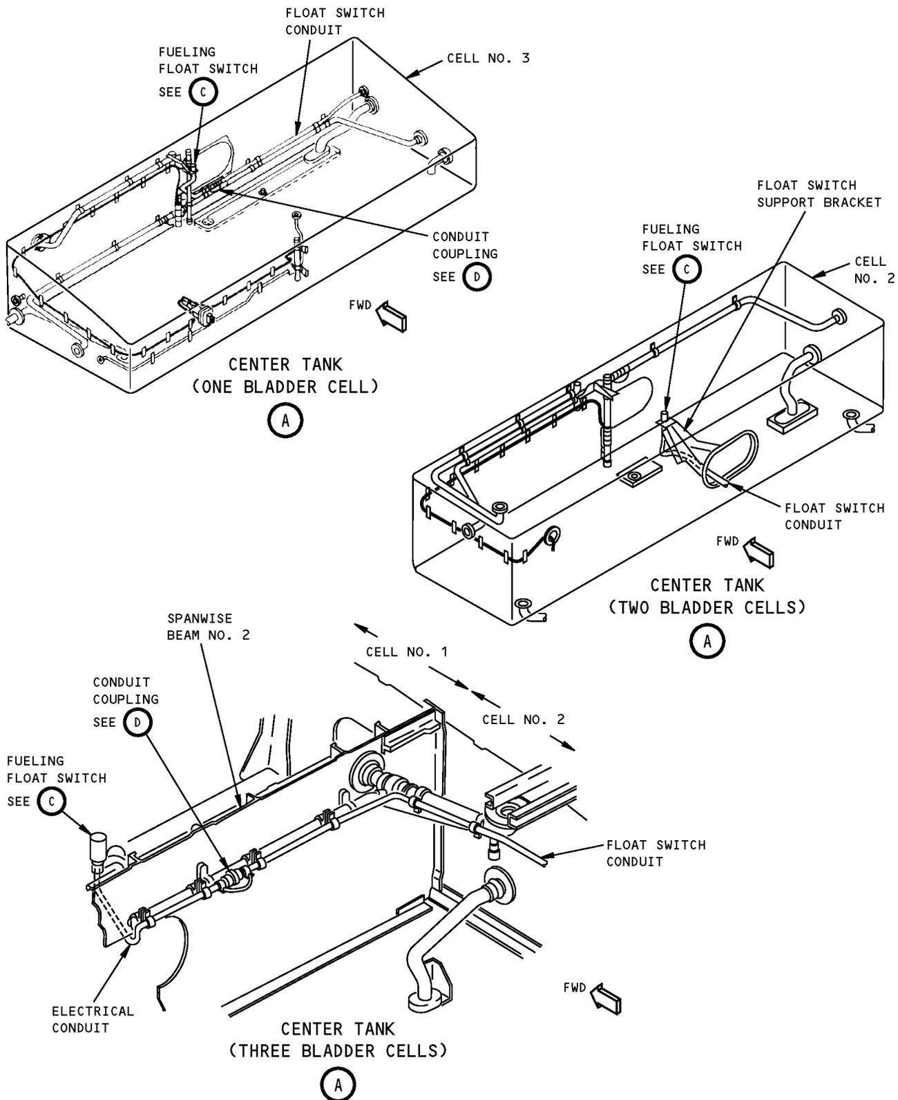
Center Tank Float Switch Installation (Type II)
