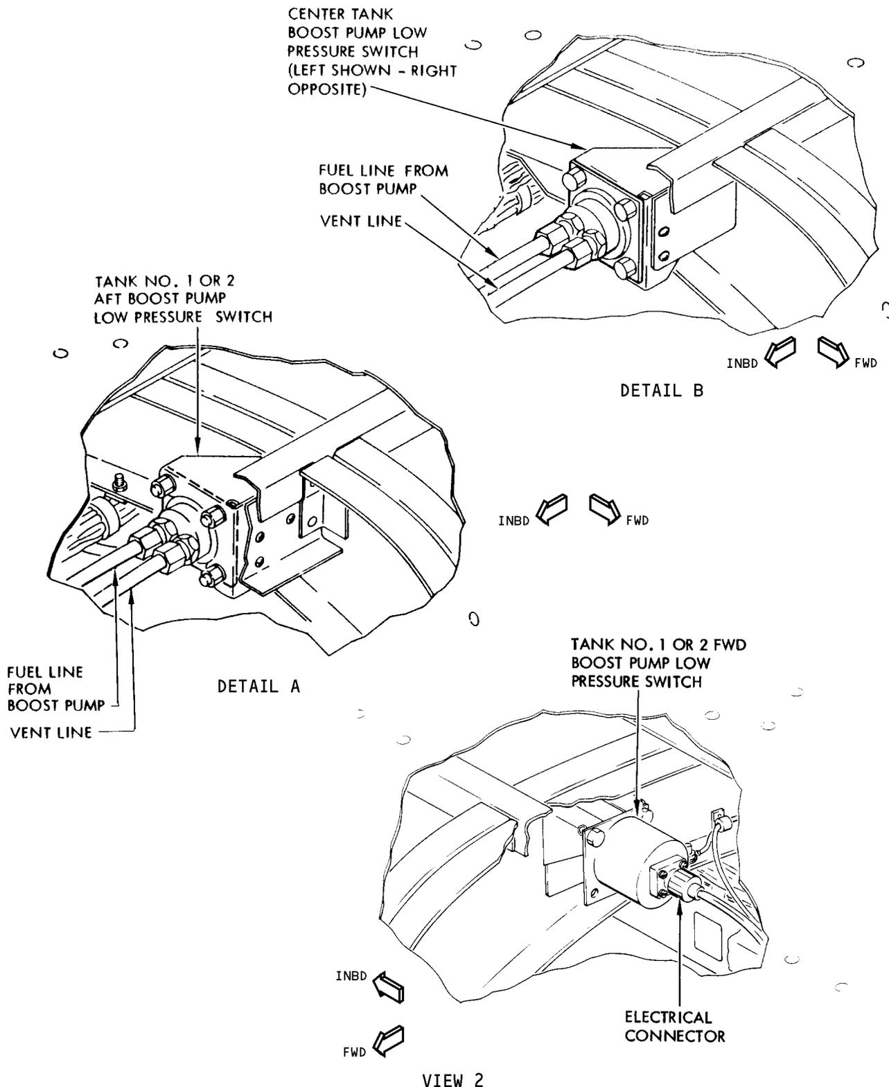
Fuel Feed Low Pressure Indicating System Component Location
