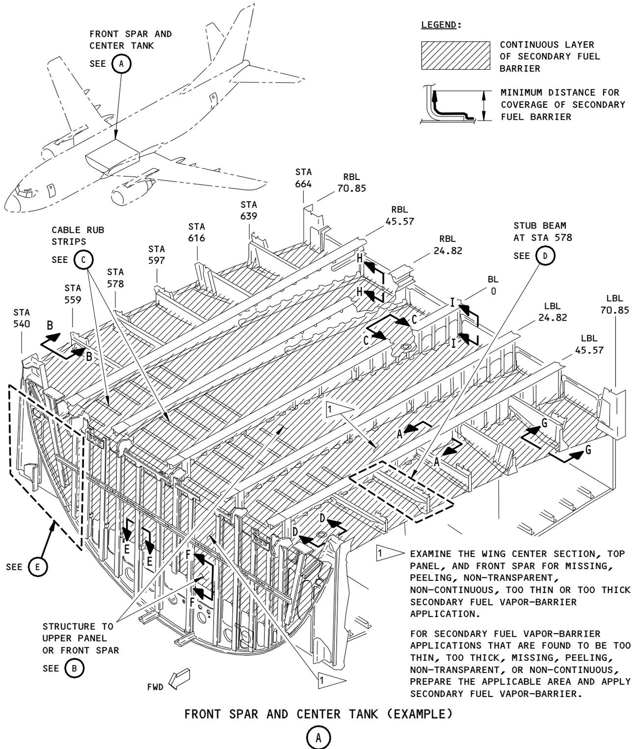
FRONT SPAR AND CENTER TANK (EXAMPLE)
