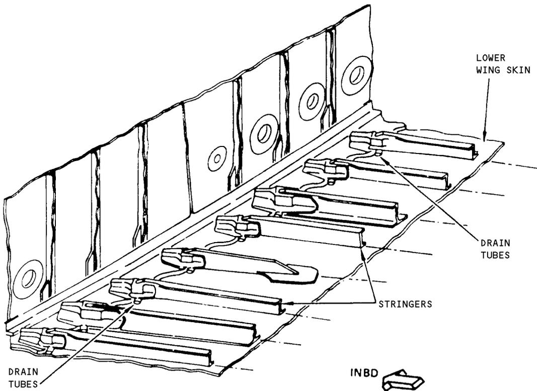
Stringer Splice Fitting Drain Tubes
