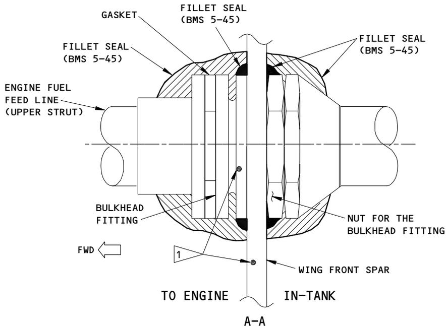
1 RESISTANCE FROM BULKHEAD FITTING TO SPAR
