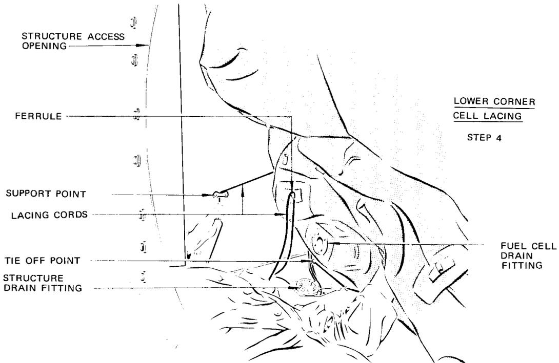
Fuel Cell Unfolding and Lacing
