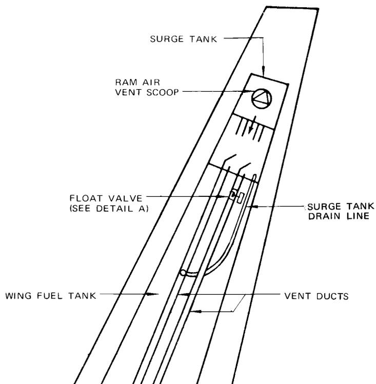
Fuel Vent Float Valve Installation
