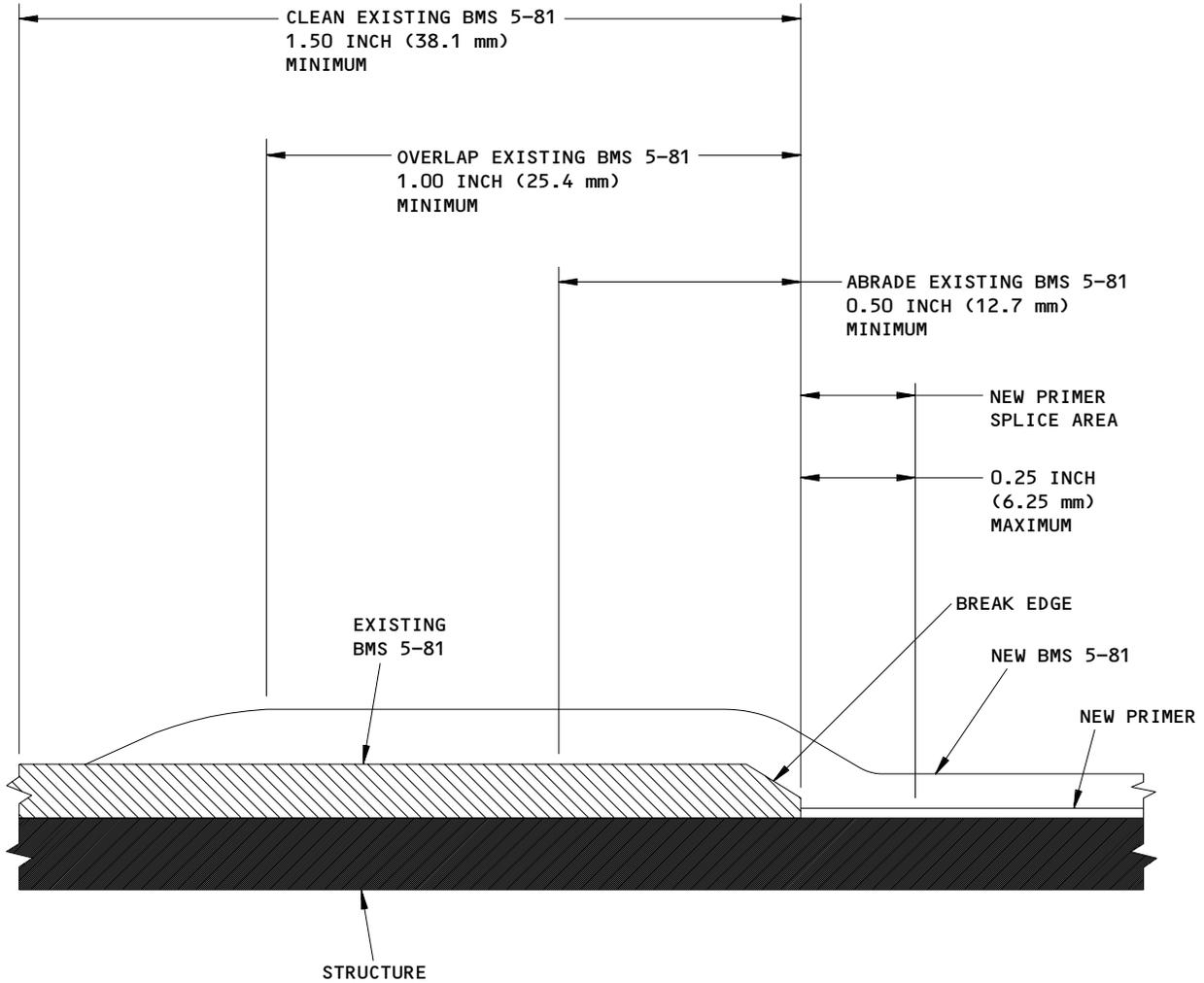
Splice Surface Area Preparation Secondary Fuel Barrier
