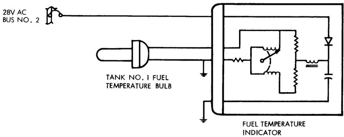
Fuel Temperature Indicating System Circuit
